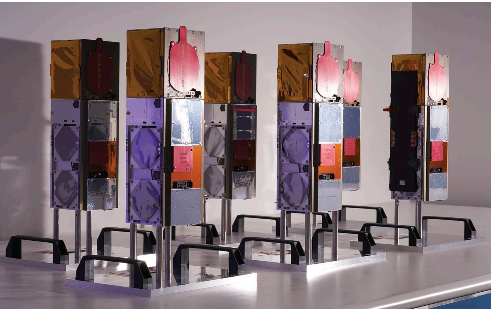
The six TROPICS satellites pictured here will be launched in 2022. Lincoln Laboratory led the program's development, and designed and built the microwave radiometer (the gold-foiled cube) at the top of each satellite. Image: Blue Canyon Technologies
