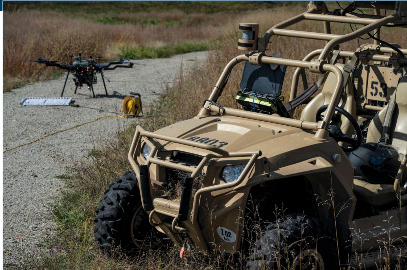
An ongoing project with the U.S. Army's Ground Vehicle Systems Center is to pair autonomous ground vehicles, such as the MRZR ATV seen here, with autonomous unmanned aerial vehicles (UAVs), like the Kraken UAV shown in the background, to improve the ATV's off-road navigation.
