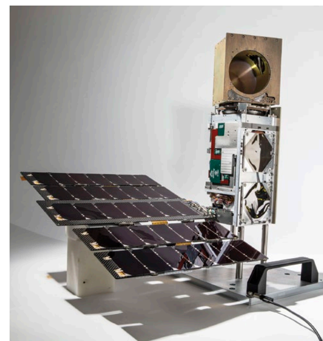
The TROPICS Pathfinder satellite pictured here entered orbit in June 2021 and successfully tested the technology, communication systems, data processing, and data flow in advance of the constellation's full launch. Image: Blue Canyon Technologies
