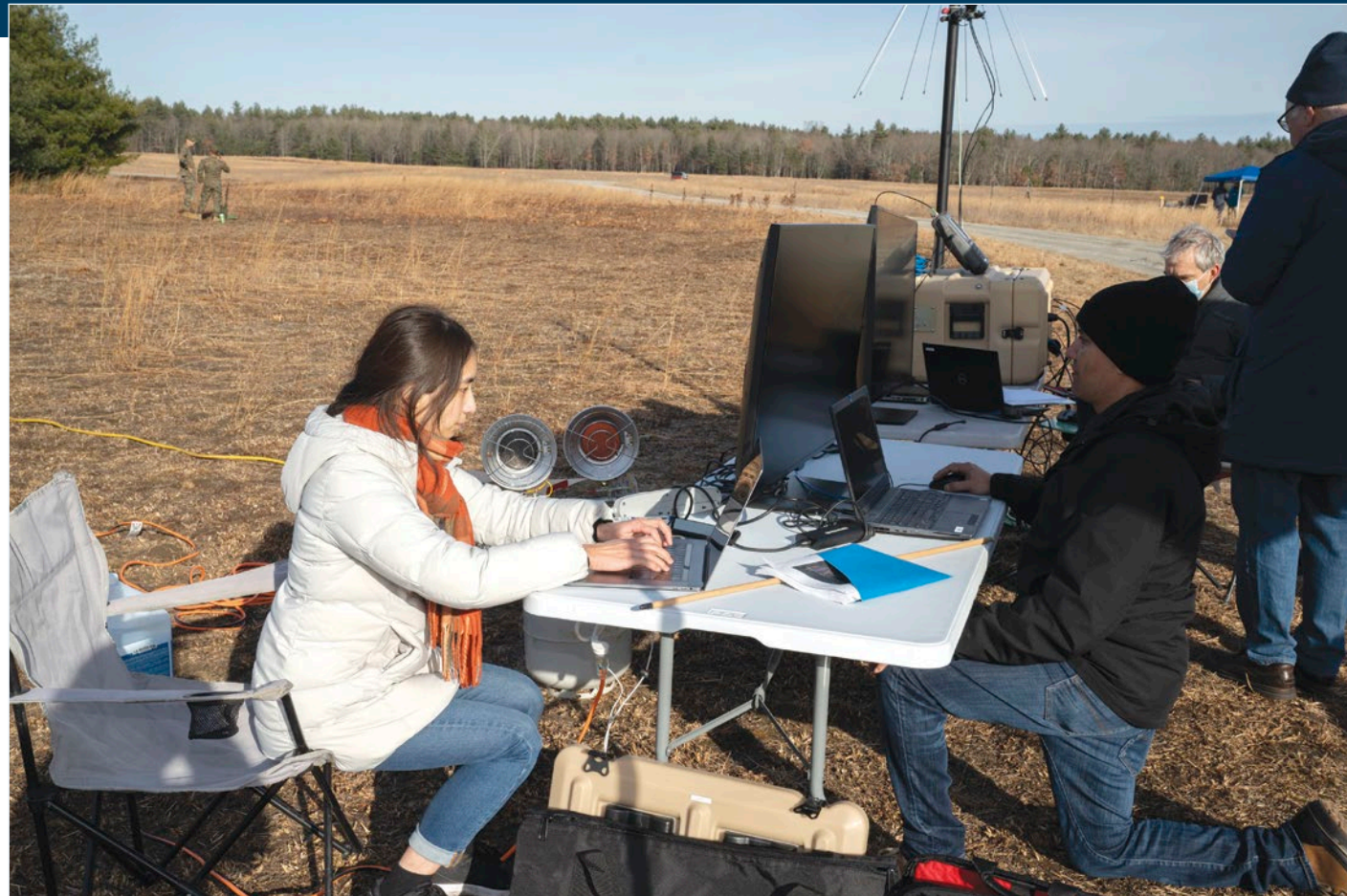
Researchers working on a Navy project showcased their automated waveform classification prototype at Fort Devens, Massachusetts. The prototype uses generative and discriminative machine learning algorithms to detect and classify RF signals.
