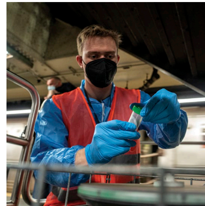
Above, at one of 120 sites in New York City, Laboratory researcher Christian Vanderloo collects filters containing samples of airborne particles. Below, Laboratory engineers designed this filter head to rotate through eight filters, eliminating time spent revisiting collection sites to replace used filters. A vacuum sucks air through each filter, trapping particles for analysis.
