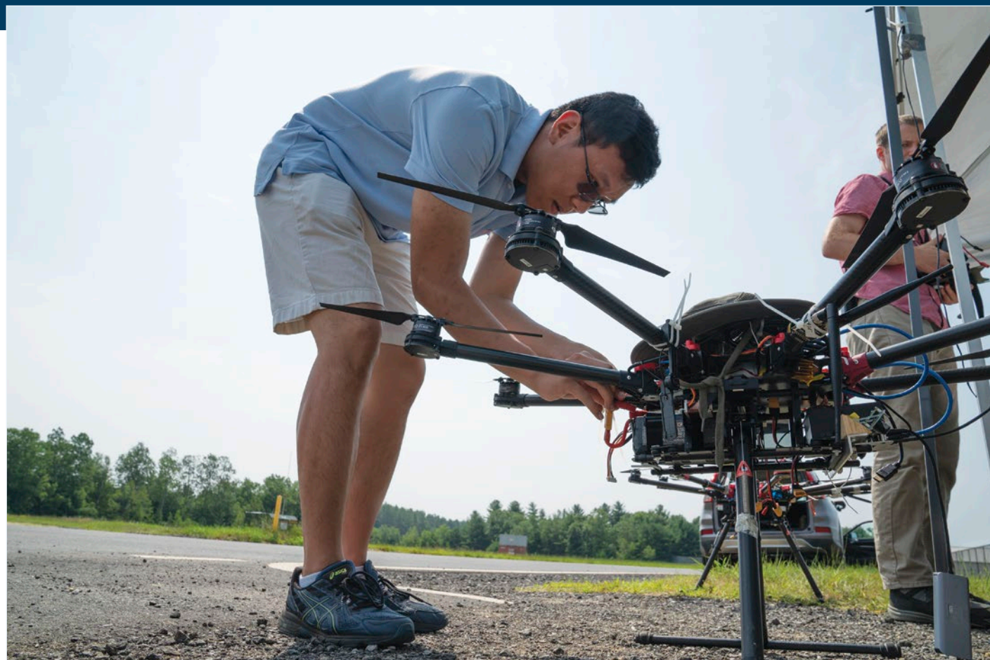
Lincoln Laboratory developed an airborne edge computing test bed to develop autonomous unmanned aircraft system (UAS) functions for homeland security missions. Above, the team field tested a “chase” UAS that autonomously follows a threat drone back to its point of origin to locate the controller.
