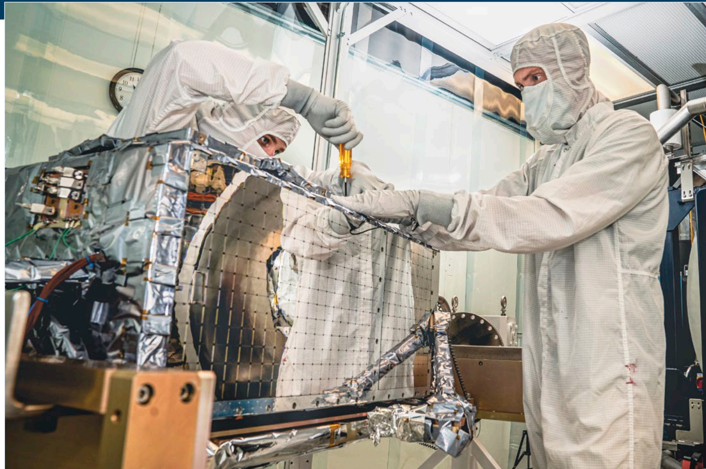
Researchers prepare one of the two Situational Awareness Camera Hosted Instruments (SACHI) for thermal vacuum testing. Each SACHI payload measures 45 x 31 x 19 inches and weighs 154 pounds.
