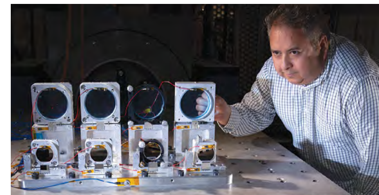
Many high-value missions rely on optical systems that must maintain precise alignment in harsh conditions. Laboratory staff have devised a patent-pending optical mount that is both easily manipulated and robust, a combination not found in commercial or commonly used custom solutions. The technology is named for its essential features: adjustable, relockable, ruggedized, and kinematic (ARRK). Shown above, engineer Andrew Guzman measures angular stability of ARRK optical mounts on a vibration shaker table.
