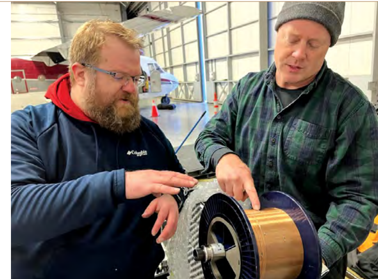
Lincoln Laboratory's Ben Evans (left) and Dave Whelihan deployed this spool—featuring 230 feet of polymer fiber with embedded temperature and depth sensors—in the Arctic. Photo: U.S. Navy Lt. Seth Koenig
