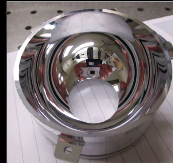
The baffle is an aluminum part created with a diamond turning machine. The fabrication process makes the baffle a precise, spherically smooth surface that does not scatter or reflect incoming light in the wrong directions. The left image shows the machined baffle prior to coating; the right shows it after coating.
