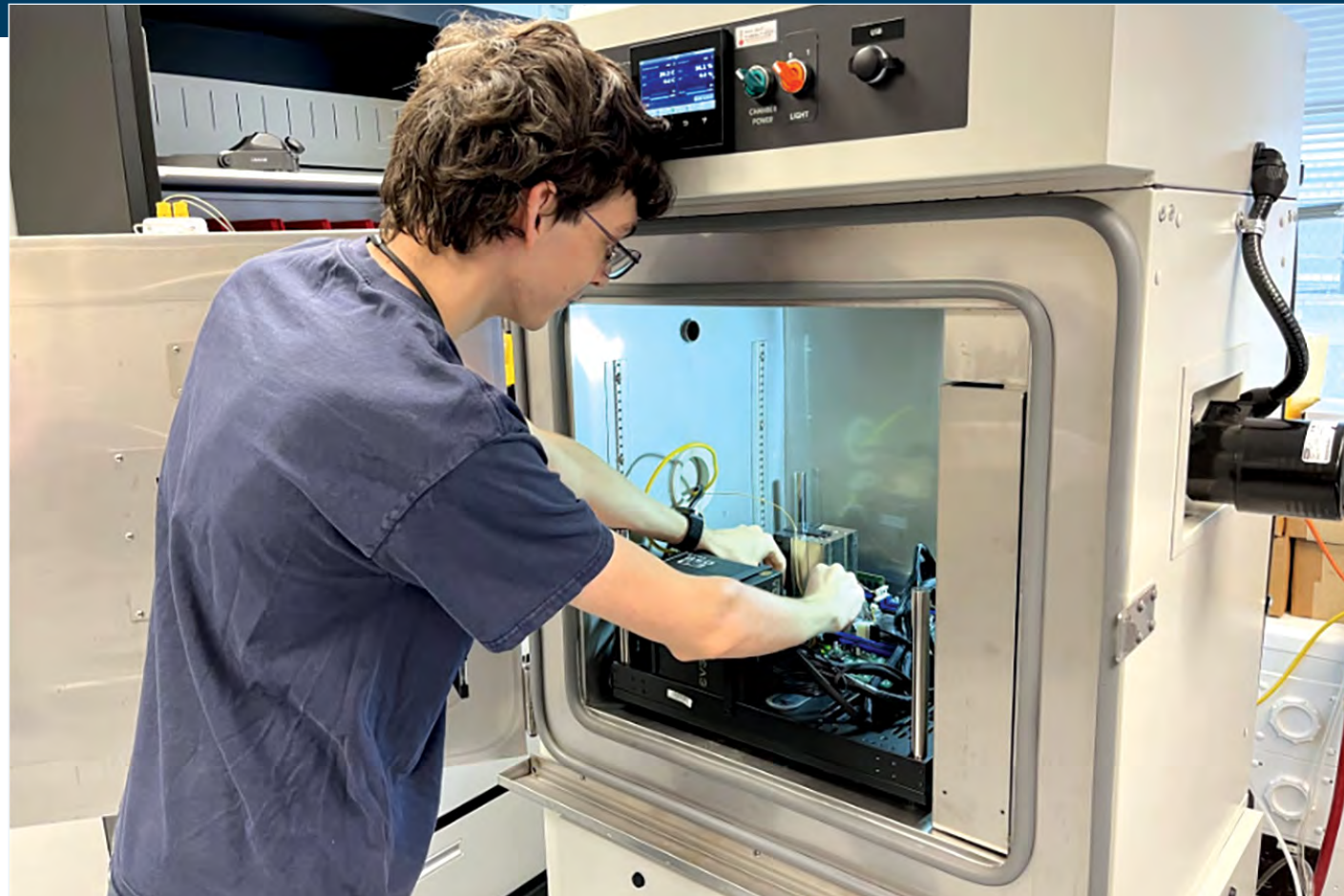
Cyber researcher Brandon John prepares an experiment to demonstrate environmental effects on security primitives within a circuit as part of the Hardware Security Analysis Testbed. These tests show how both temperature and humidity can affect the operation of encapsulated integrated circuits.
