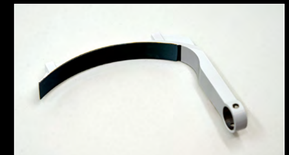
The occulter, shown here, is fabricated from aluminum following the same process used on the baffle.
