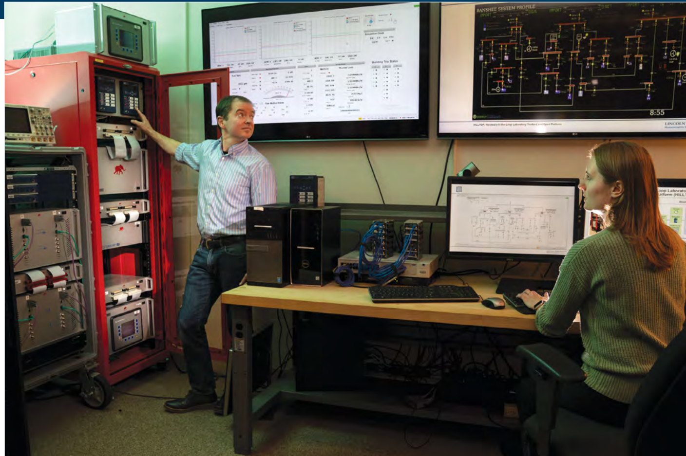
Nicholas Judson and Jean Sack test new control algorithms for the Hardware-in-the-Loop Laboratory Testbed and Open Platform. The platform acts as a digital twin to energy control systems, simulating loads and enabling operators and researchers to assess the vulnerabilities and defenses of their systems.
