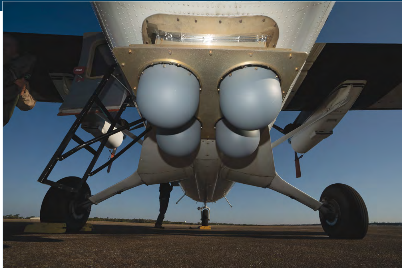
The four radomes on the test aircraft above house phased array antennas that automatically form multiple transmit and receive beams to link nodes in a scalable airborne mesh network. This aircraft enables evaluation of new communication waveforms, networking protocols, and sensing approaches.
