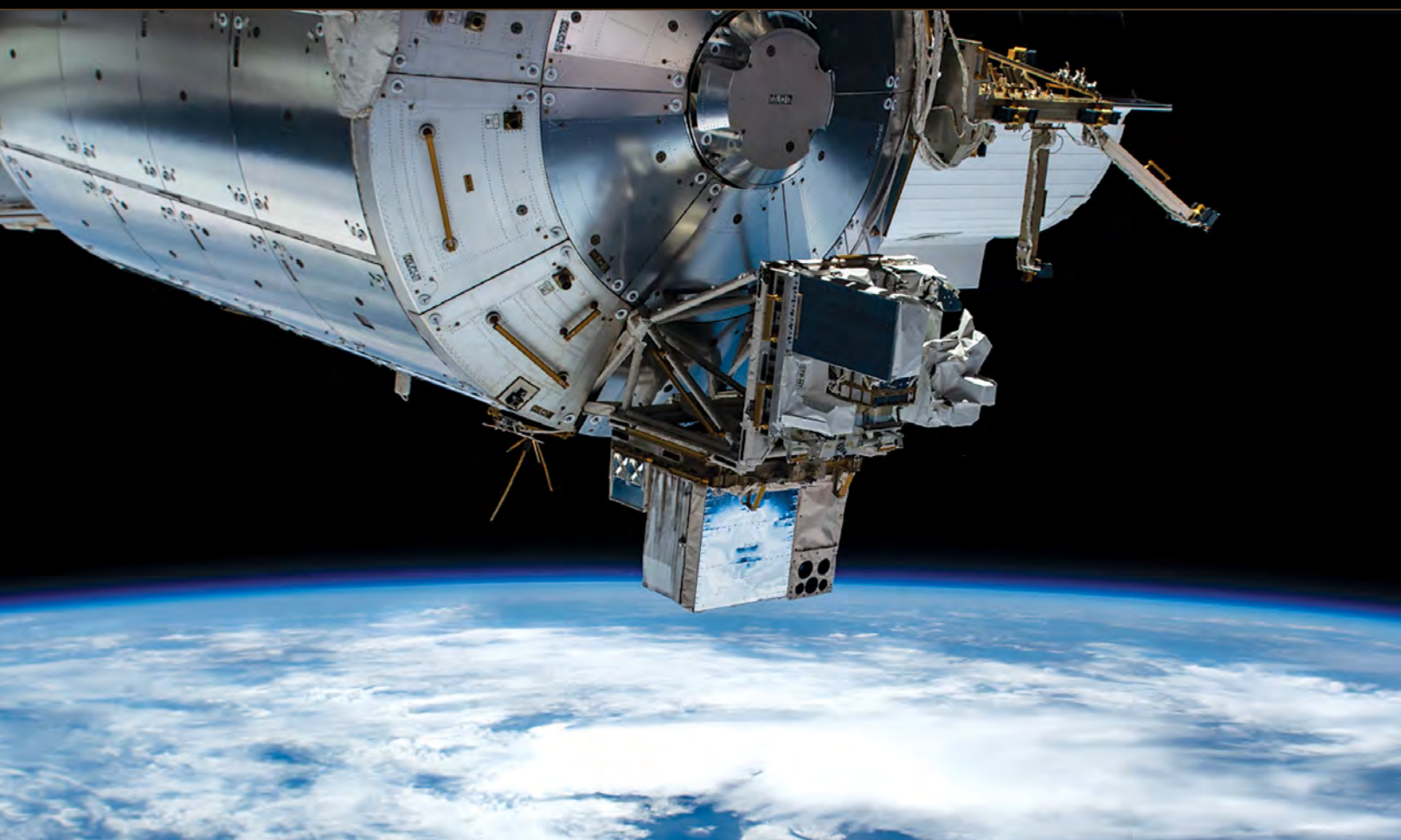
The Local Area Space Situational Observations hardware can be seen attached to the International Space Station. The data from its mission will help inform the future of solar occlusion in space. Photos by the Space Test Program, Houston Office
