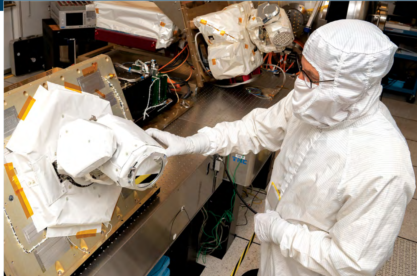
Here, staff member John Wellman inspects the optical communication terminal built for NASA to demonstrate 1.2-gigabits-per-second data transmission from the International Space Station to a ground station via the Laser Communications Relay Demonstration satellite launched in December 2021.
