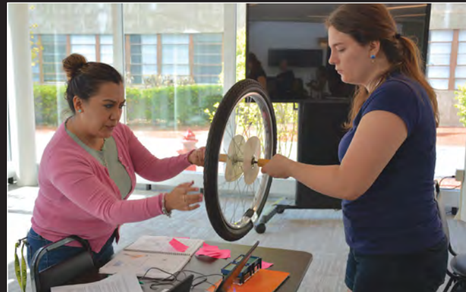
Esmeralda Hernandez (left) and Liz Raine spin a wheel above a small self-built radar system to determine the wheel’s speed based on the Doppler effect.
