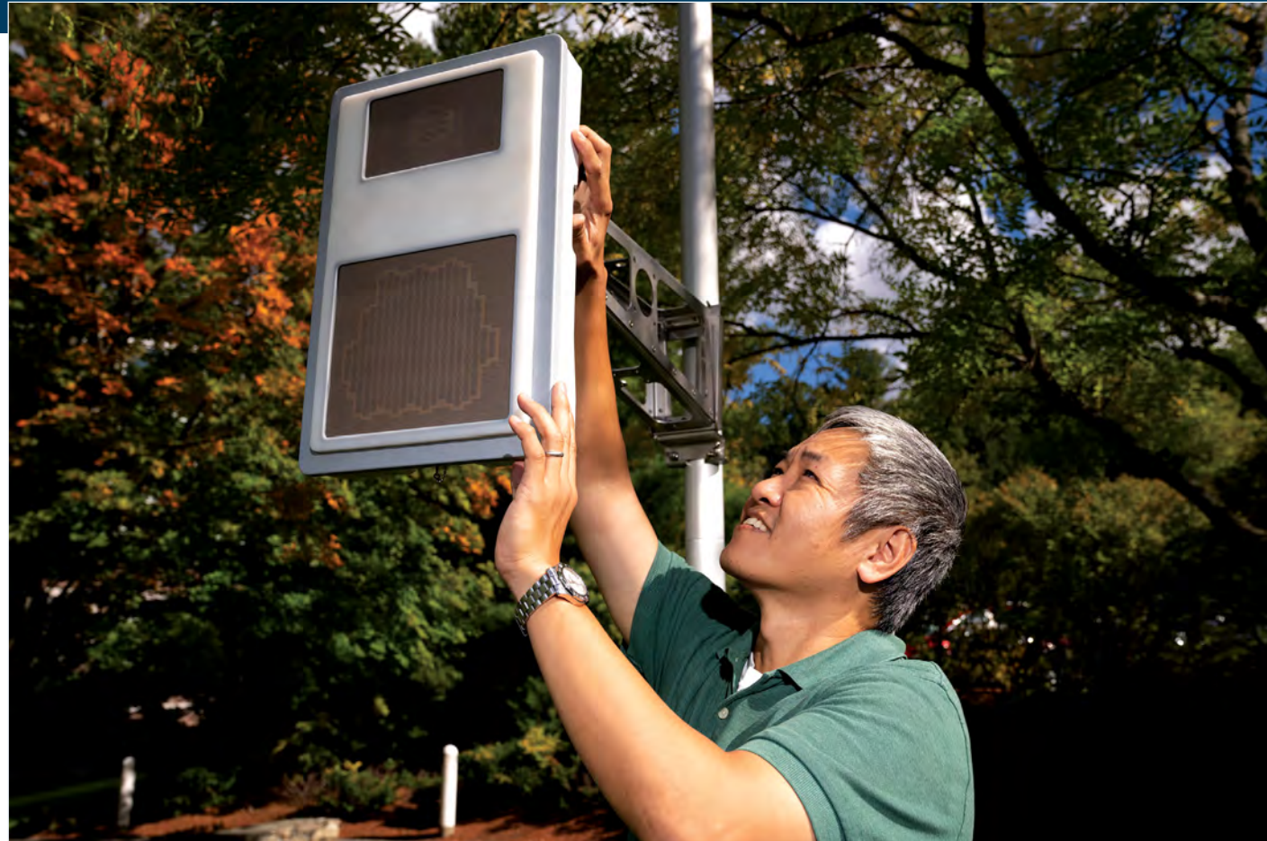
The Laboratory is evaluating surveillance technologies to support small uncrewed aircraft system operations. Here, staff member Tan Trinh configures a primary radar proposed for use by the Massachusetts Department of Transportation to enable drone-based airborne rail inspection.
