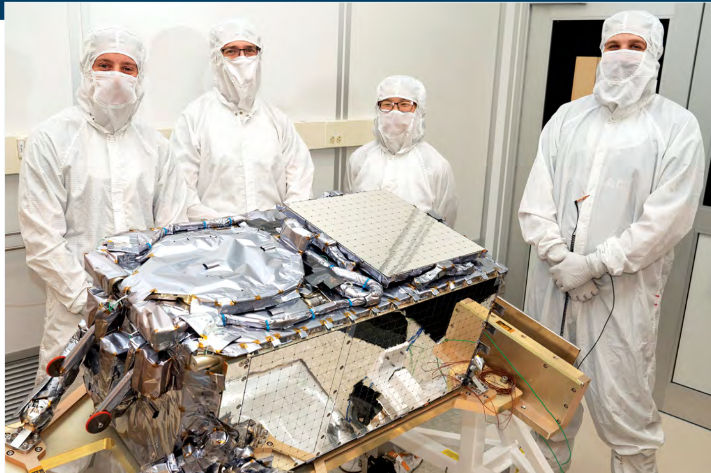
The Situational Awareness Camera Hosted Instrument space domain awareness sensor payloads will be hosted aboard two Japanese satellites launching in late 2023 and early 2024. Each payload, one of which is pictured above, measures 45 x 31 x 19 inches and weighs 154 pounds.
