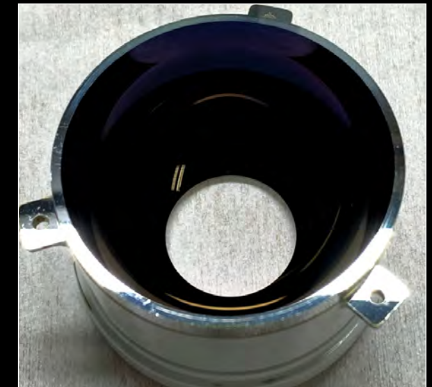
The baffle is an aluminum part created with a diamond turning machine. The fabrication process makes the baffle a precise, spherically smooth surface that does not scatter or reflect incoming light in the wrong directions. The left image shows the machined baffle prior to coating; the right shows it after coating.
