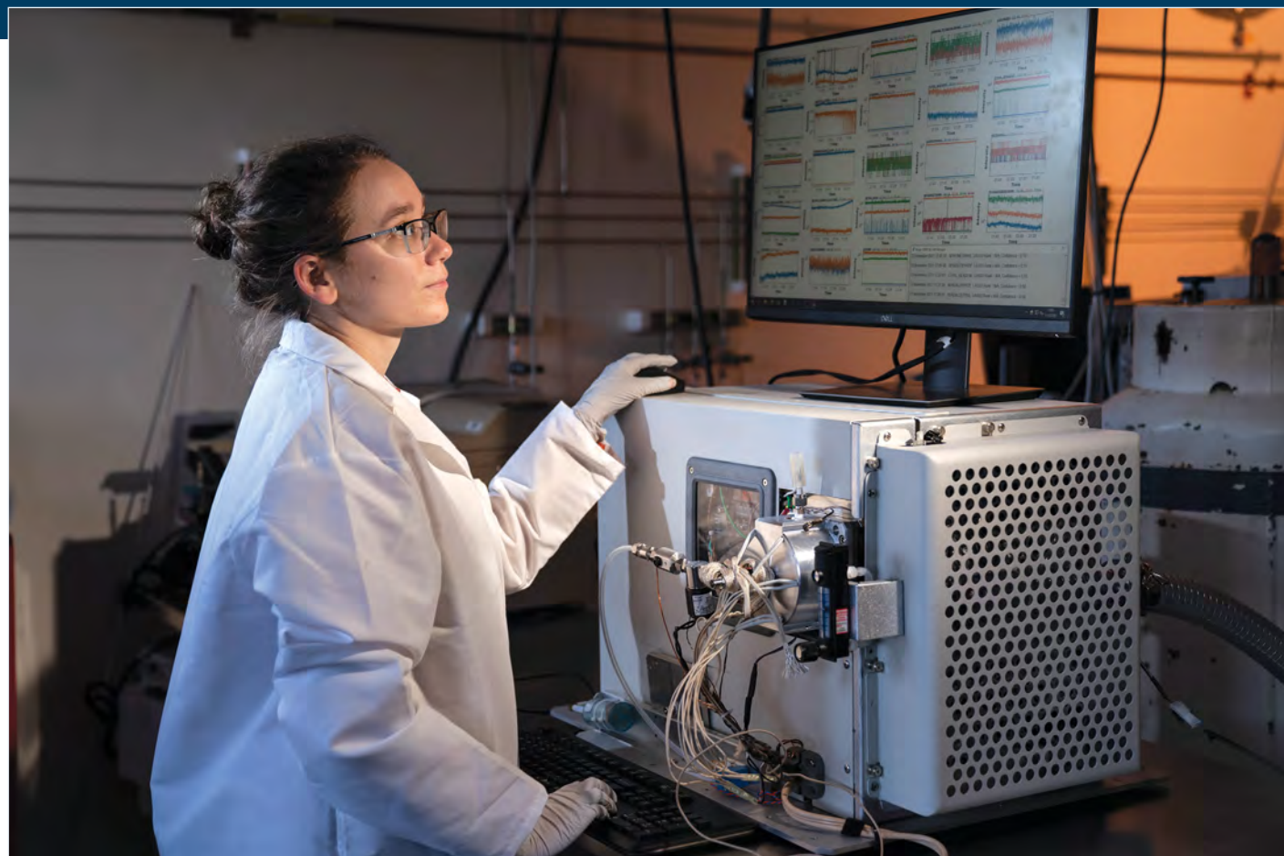
Lincoln Laboratory worked with an industry partner to develop a ruggedized, transportable triple-quadrupole mass spectrometer for collecting hyper-localized, highly specific chemical data. Here, Alexandra Wrobel calibrates the device prior to deployment.
