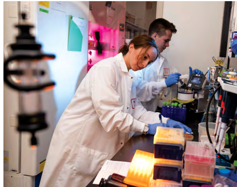
Researchers Arianna Comendul and Victor Cabrera prepare emulsion reactions to characterize antibody-target binding events. Within each water-in-oil emulsion droplet, DNA encoding the antibody and target are joined and amplified, and the product from all droplets is pooled and sequenced. These experimental results will be used to train AI algorithms to predict what antibody sequence is likely to bind to a new target, with the goal of enabling the rapid creation and optimization of therapeutic antibodies.
