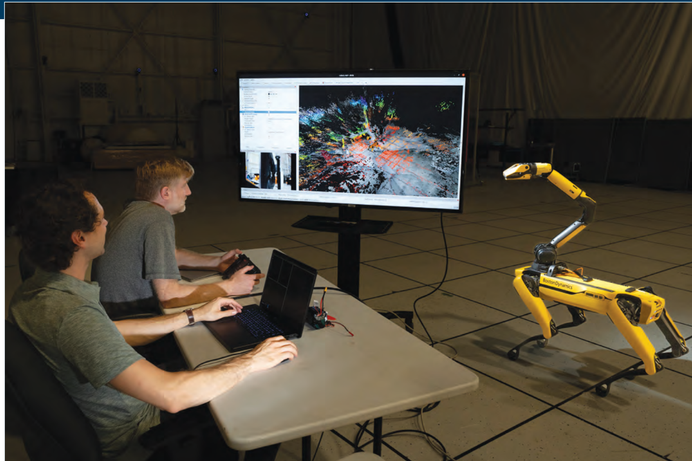
Using Boston Dynamics' Spot robot, Eric Cristofalo, left, and Dan Griffith test a real-time, hierarchical, indoor, sparse-mapping algorithm called Hydra. The advanced algorithm supports complex navigation with very low-size, weight, and power requirements.
