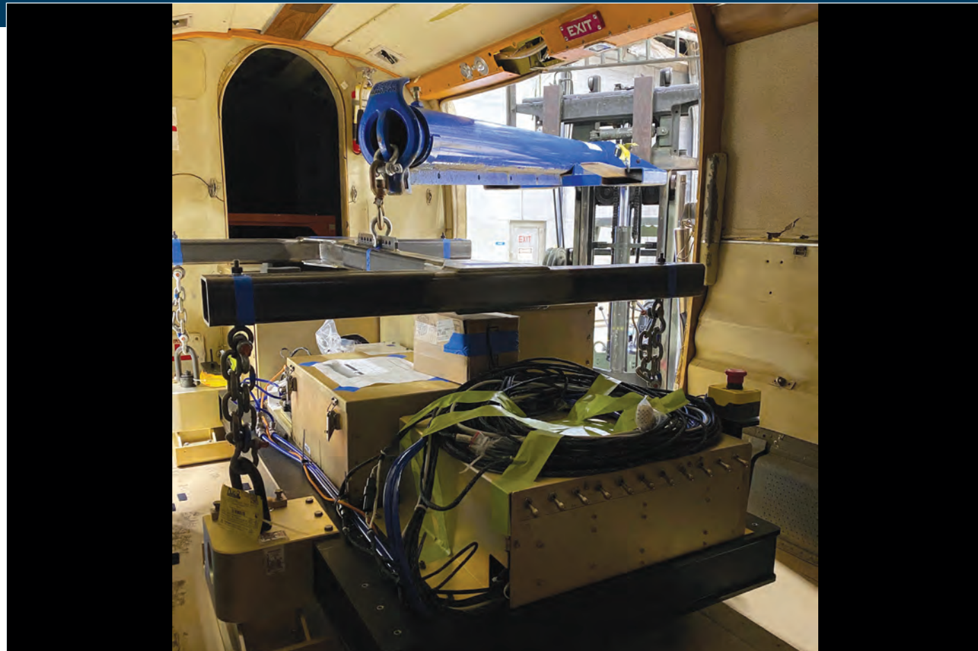
PHOENIX High CASTLE—a next-generation photon-counting 3D imaging lidar sensor funded by the U.S. Army Engineer Research and Development Center's Geospatial Research Laboratory—is hoisted into the Army C5ISR (Command, Control, Communications, Computers, Cyber, ISR) aircraft.
