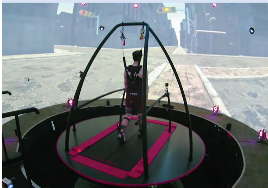
A study participant wearing an exoskeleton approaches a yellow light within a simulated city intersection.
