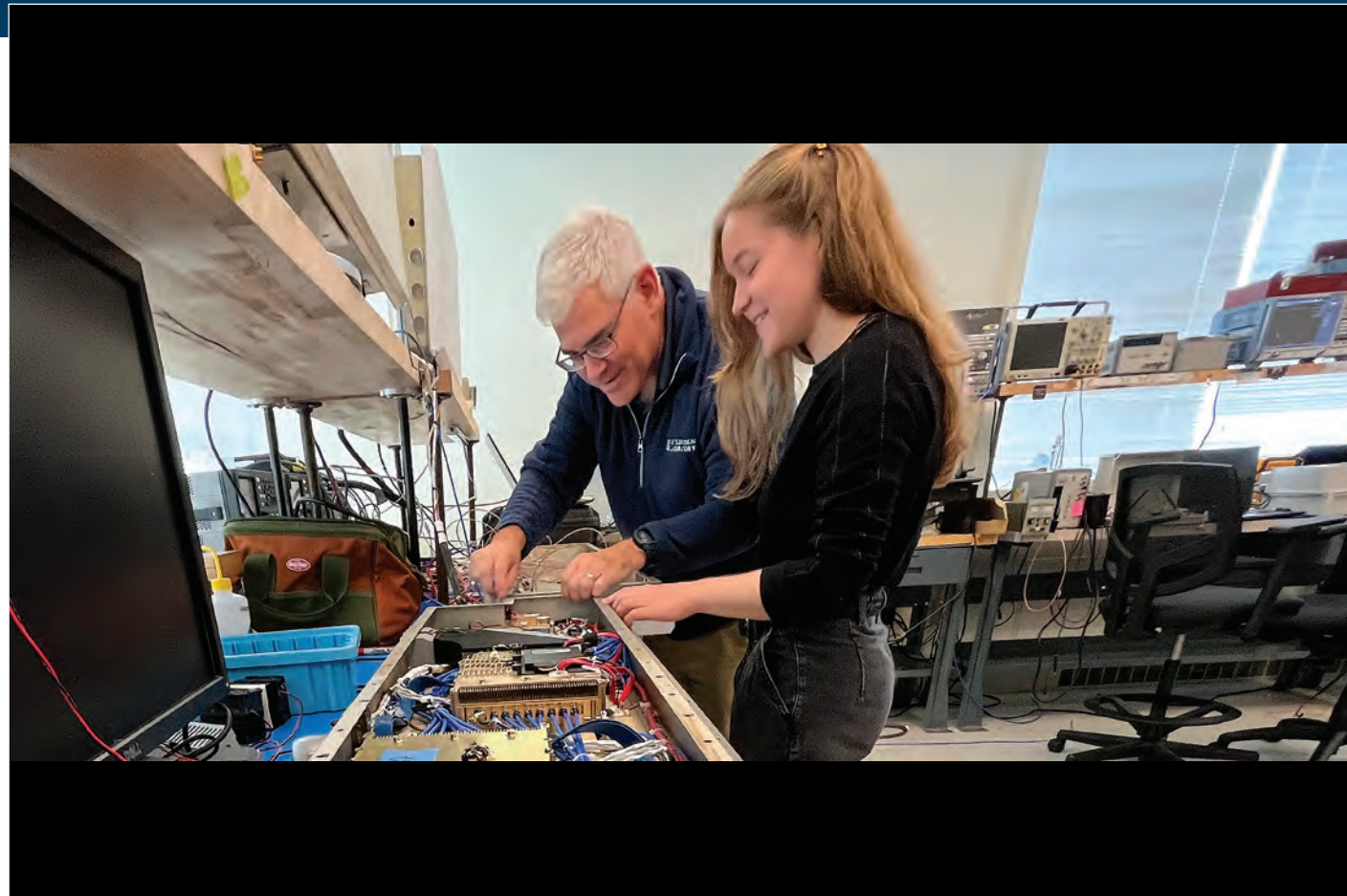
Melinda Burns, front, and Richard Gentile inspect an RF sensor to be loaned to a U.S. government sponsor for use in theater. This prototype unit builds on the hardware and processing architecture developed in recent years by the Lincoln Experimentation and Novel Technology Innovation Lab team.
