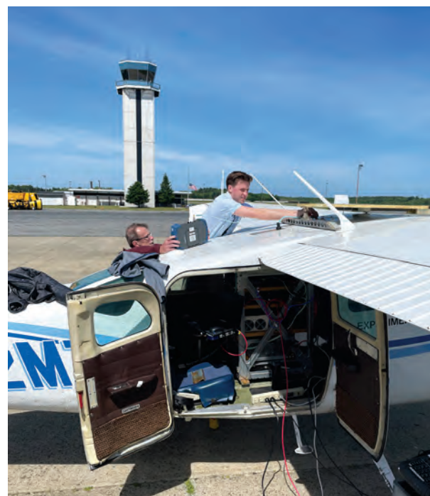
Above, William O’Connell, left, and Nicholas Winicki install and test a small platform radio in a Cessna 206 for air-to-air communications. Below, the Saab aircraft outfitted with the ARTB takes off.
