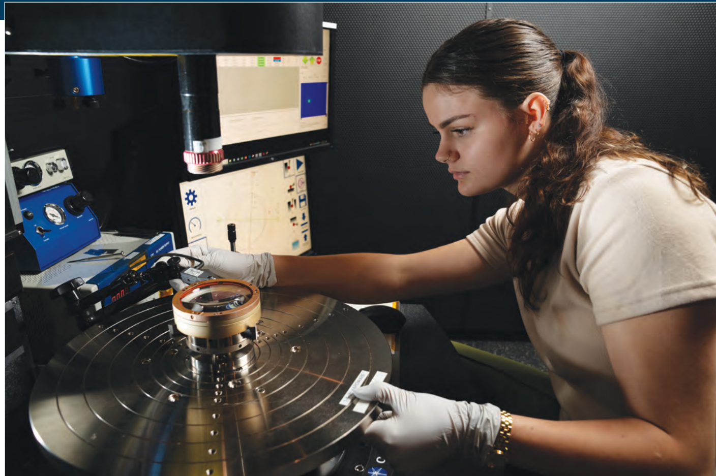
The Laboratory has developed a compact hyperspectral spectrometer that achieves state-of-the-art optical and signal-to-noise performance while being significantly smaller than existing spectrometers. Here, Bayleigh Nugent aligns an optical element for the hyperspectral imaging spectrometer.
