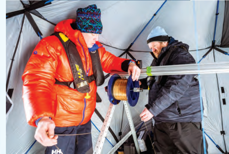
Above, David Whelihan, left, and Benjamin Evans inspect a spool of fiber embedded with temperature and depth sensors before they lower the spool into the water. At left, Lincoln Laboratory and GLRC researchers test locations for data collection on Huron Bay ice. Photos: GLRC
