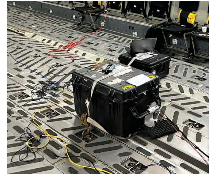
MagNav equipment (contained in the black boxes) and a laptop are loaded on the back of a C-17A Globemaster III. The system successfully positioned an aircraft within a magnetic map.
