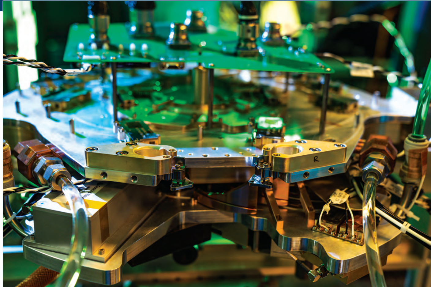
The Advanced Sensor Technology Ruggedized Integrated Experiment program demonstrated a novel, highly capable ruggedized fiber-laser prototype, pictured above, suitable for future air- or space-based sensing applications.
