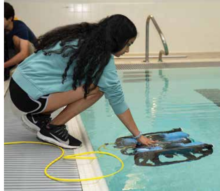
A student in the AUV Challenge course submerses her programmed AUV to test its ability to navigate through an underwater obstacle field.
