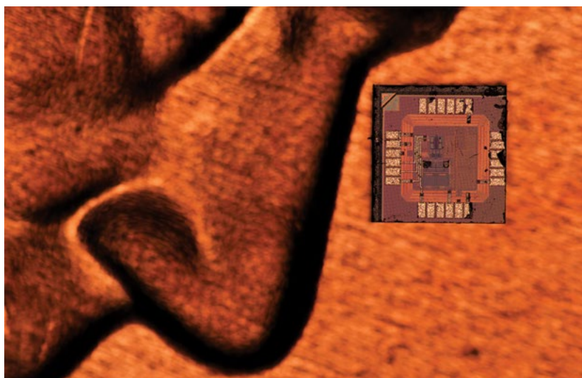
The application-specific integrated circuit, or ASIC, responsible for sensing voltage spikes in the brain is photographed here for scale on the face of a penny, next to Lincoln's nose.
