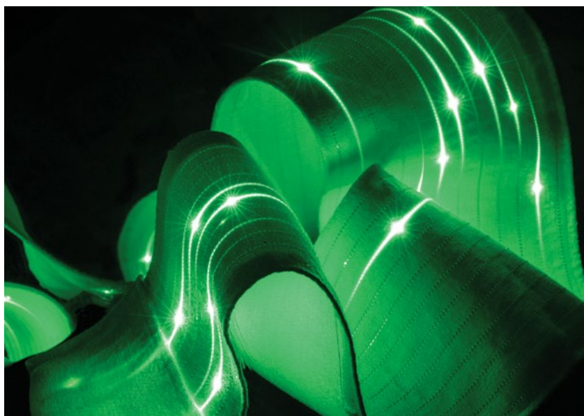
Fibers drawn from a preform with embedded LEDs are woven into fabric by using a conventional weave.
