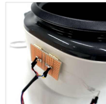
An infrared sensor measures the temperature of food inside a rice cooker, triggering a controller to shut off power when a certain temperature is reached.
