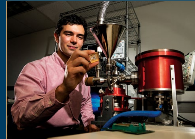
Demonstration of a germanium CCD with sensitivity that spans from the visible through the shortwave infrared and that has enhanced sensitivity to hard X-rays. Here Michael Collins tests a germanium CCD in a cryostat.
