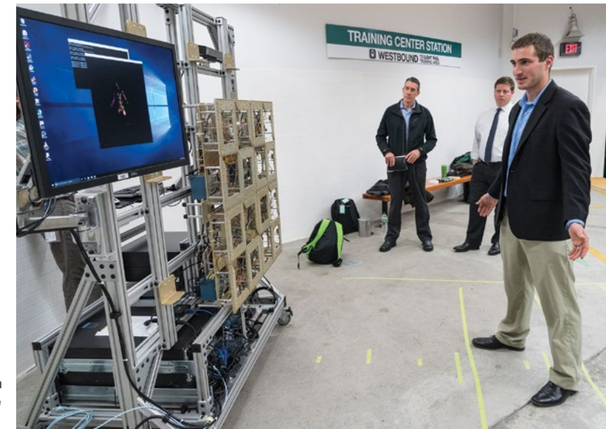
Above, the Laboratory's prototype microwave imaging system identified a metal can inside the subject's backpack. At right, Lincoln Laboratory researcher William Moulder is scanned by the microwave imaging system when it was tested at a transportation center.
