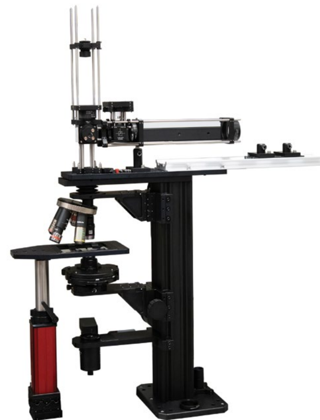
Laboratory engineers designed this hyperspectral and quantitative phase imaging microscope. Using these two imaging methods, researchers may study and quantify tissue structures without needing to apply various stains to the sample.
