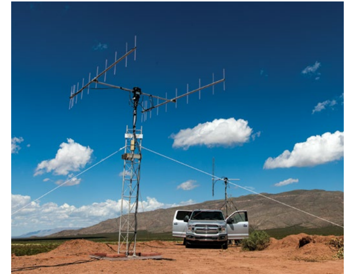
For the testing, four ground terminals were configured across New Mexico, demonstrating the system's capability over ranges spanning hundreds of kilometers. High-gain receive antennas, such as the one above, were part of the ground terminal setup.
