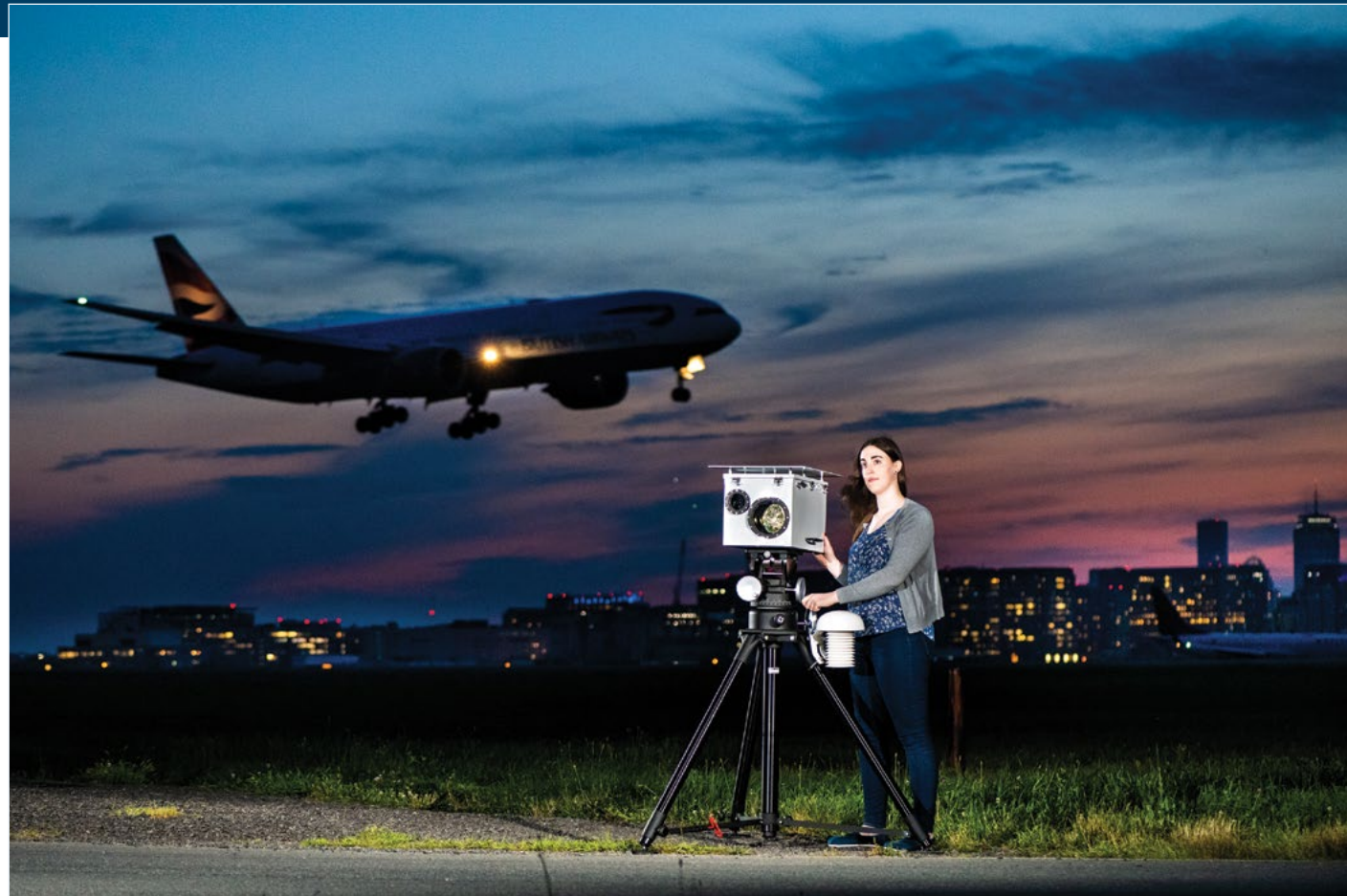
Laboratory staff tested a prototype system at Boston Logan International Airport; the system allows law enforcement to rapidly locate individuals who are using handheld lasers near airports to disrupt the vision of pilots in flight.
