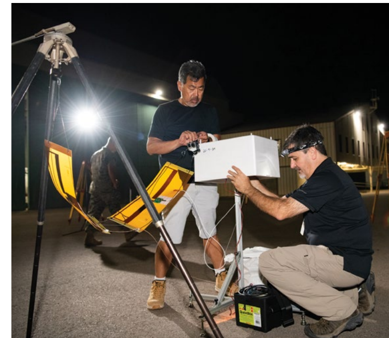
Before sunrise, team members began preparing the 12 balloon payloads that launched from Roswell, New Mexico. The payloads are housed in a styrofoam case with their antennas suspended to allow system checkout prior to launch.
