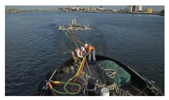
In 2021, researchers deployed a rigid frame on which a technology demonstrator undersea-mapping sparse sonar array was mounted for sea tests of the array's capability intended to provide resolution two orders of magnitude higher than currently achievable.
