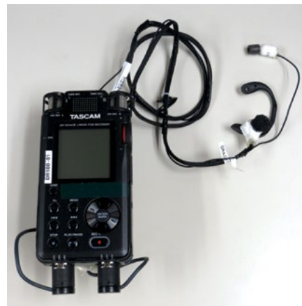
FIGURE 5. As an alternative to the second-generation dosimeter, Lincoln Laboratory augmented a commercial noise recorder (above) with dual microphones and custom housings so that it could be used during a military exercise.
