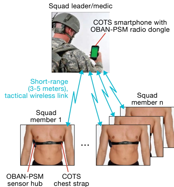
FIGURE 3. The OBAN PSM system allows team leaders or medics to monitor the current physiological status of their squads via a short-range tactical wireless link.
