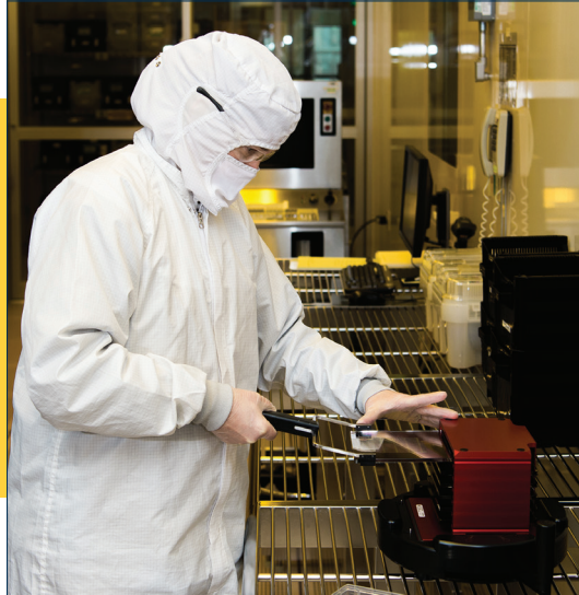
At left: A reticle is loaded into a pod for 193-nanometer lithography wafer patterning
