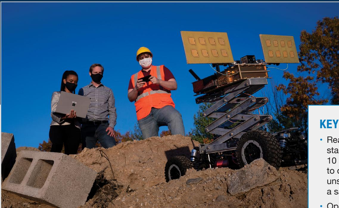
The MURMUR sensor is integrated on an unmanned ground vehicle for deployment to disaster sites. Operators remotely control the system to fine-tune its sensitivity while search-and-rescue teams see detections in real time on a mobile device.
