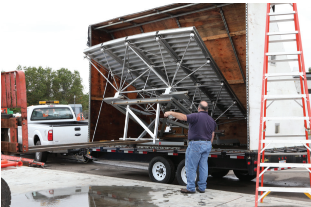
FIGURE 41. A subframe is secured to the steel frame on the transport trailer and then pivoted to fit inside the 8-foot-wide trailer body.
