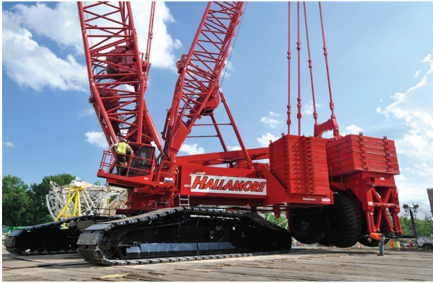
FIGURE 16. Under heavy loads, the crane's 230-ton auxiliary counterweight lifts completely off the ground.
