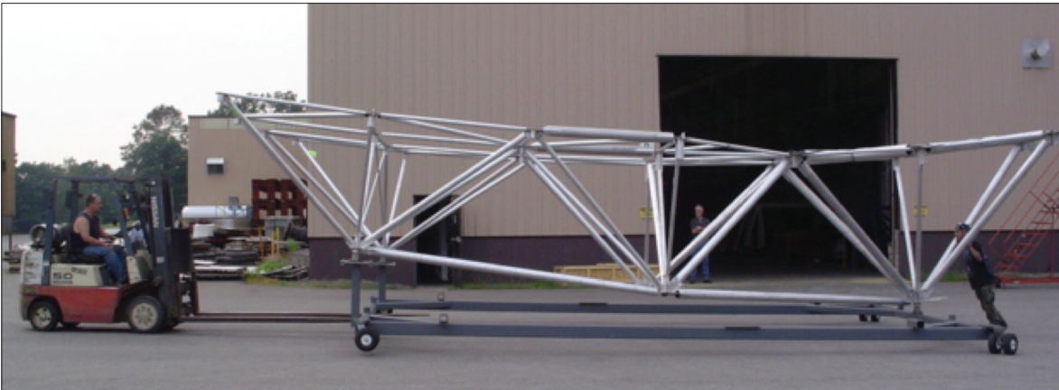
FIGURE A5. Completed radial rib assembly.
