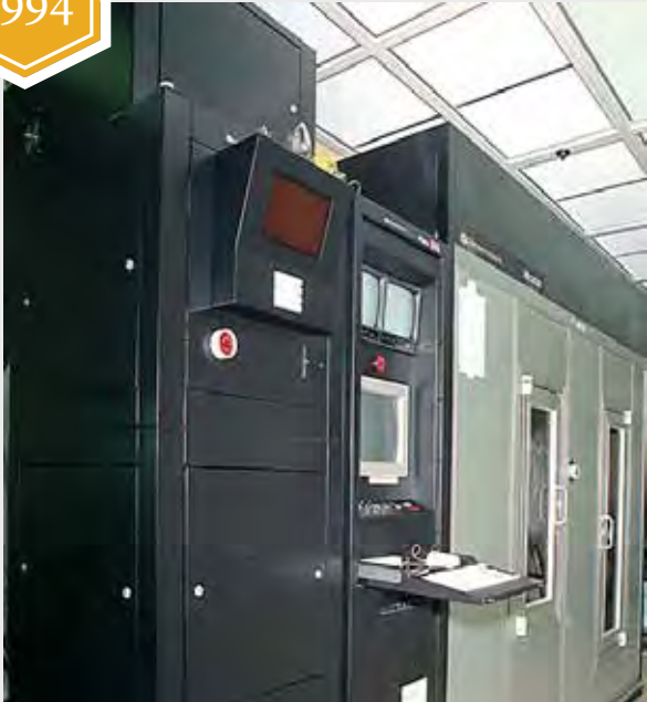
World's first 193 nm wafer exposure system in the Microelectronics Laboratory
