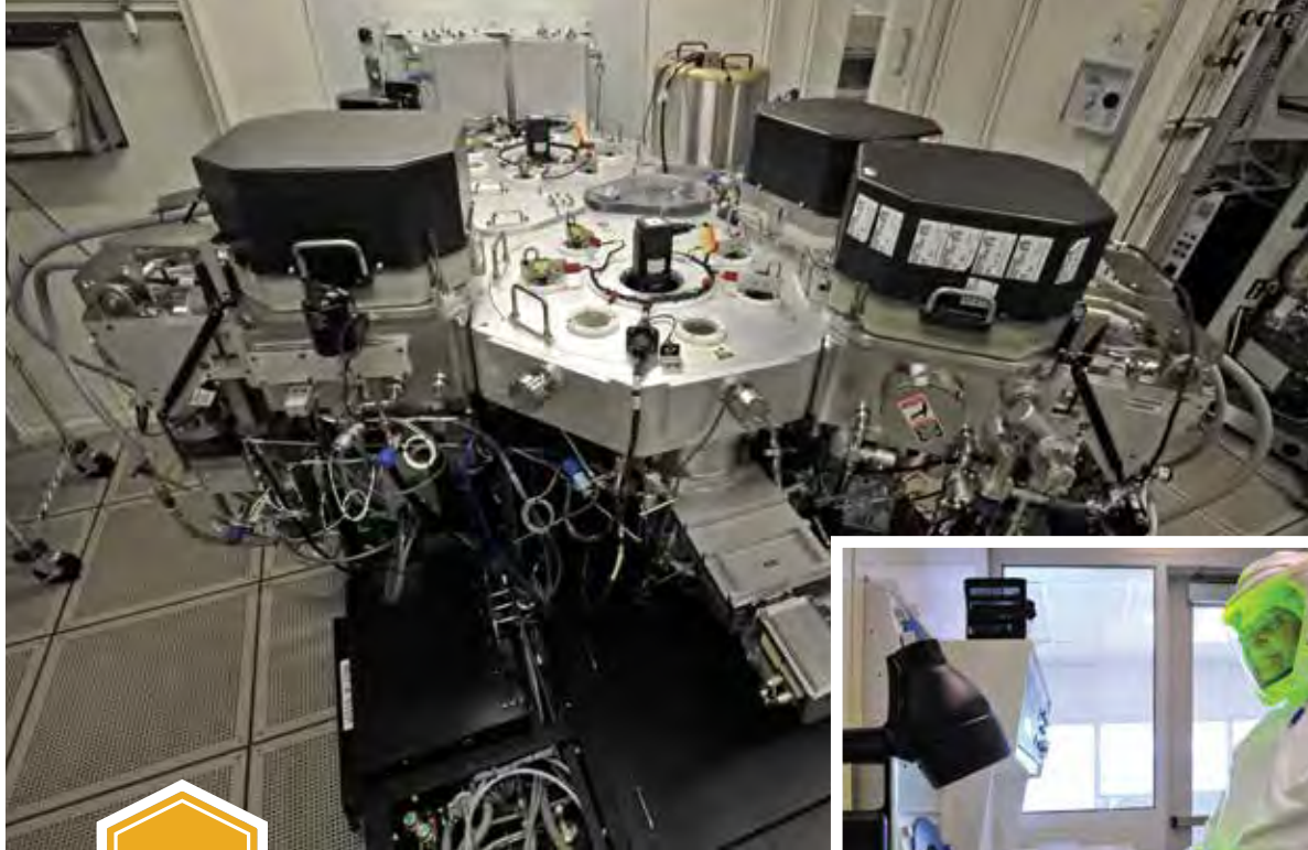
Large image, metal-deposition tools; inset, technician inspecting a wafer
