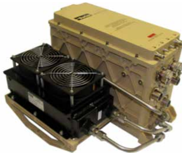
FIGURE 15. The SprayCool processing chassis offers a customizable commercial all-condition chassis with closed-circuit cooling for the internal autopilot and LGPR electronics.
