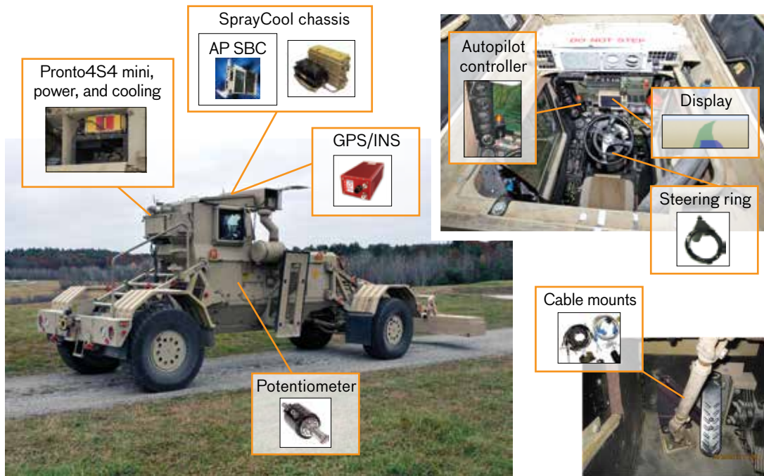
FIGURE 12. The Lincoln Laboratory autopilot system is shown installed on the Husky Mark III vehicle. In order to maintain the integrity (and safety) of the Husky, the installation of the hardware components needed to be completed with minimal modifications to the vehicle. Although components are mounted in various locations on the vehicle, the installation required only two permanent modifications—two small holes in the brake pedal.
