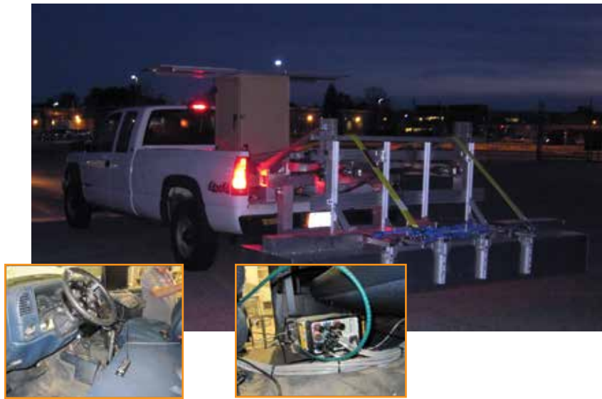
FIGURE 16. Initial testing of the autonomous system was performed on a pickup truck that used real-time kinematic GPS positioning for autonomous operation. The Pronto4 drive-by-wire system was installed in the vehicle. The LGPR unit was developed in parallel and attached on the rear of the truck as shown in the lower right. The recommended position for the Pronto4 unit (under the seat) was available here, unlike on the Husky, which required installation in an external toolbox.
