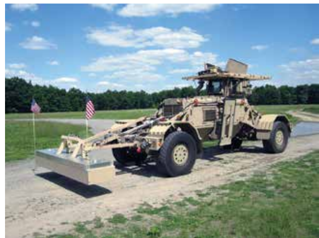
FIGURE 22. Above is an image of the Husky during the world’s first successful demonstration of LGPR-based autonomous ground vehicle operation on 31 May 2012.
