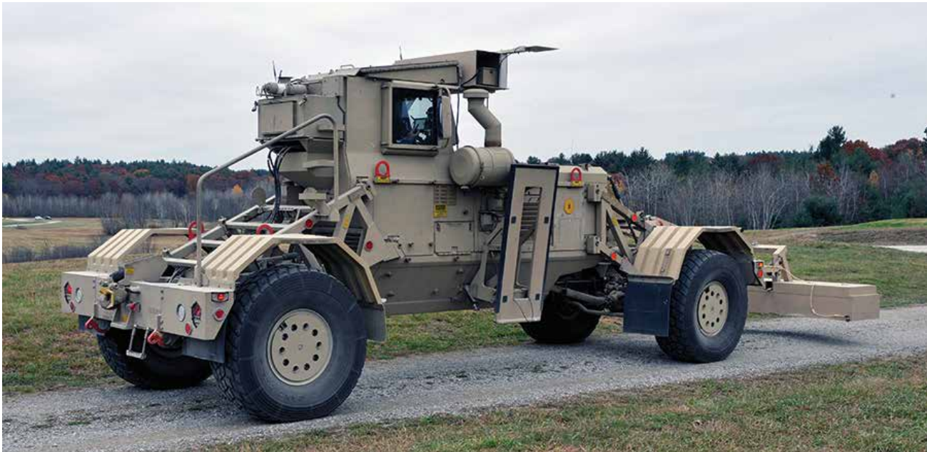
FIGURE 1. The Husky Mark III is shown with the Lincoln Laboratory autopilot and localizing ground-penetrating radar (LGPR) components installed. Autonomous LGPR-based operations were demonstrated on four Husky systems, two of which served three months of operational evaluation in Afghanistan.
