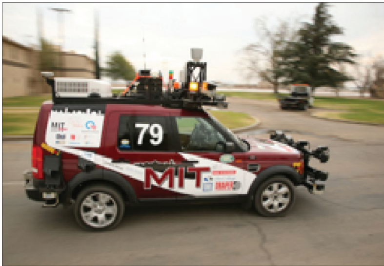
The TALOS autonomous vehicle begins a qualifying run at the DARPA Urban Challenge. Sensors scan and sweep across an intersection to show approaching and standing traffic that TALOS' algorithm must assess before continuing. Note the empty driver's seat.
