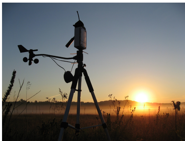
Sensor at sunrise: a grid of high-fidelity smoke detectors and collocated anemometers was tested at Fort Devens, Mass., in August 2007. Such an array of sensor nodes can monitor the smoke plume's shape and movement—information that would be critical in a biological or chemical release.
