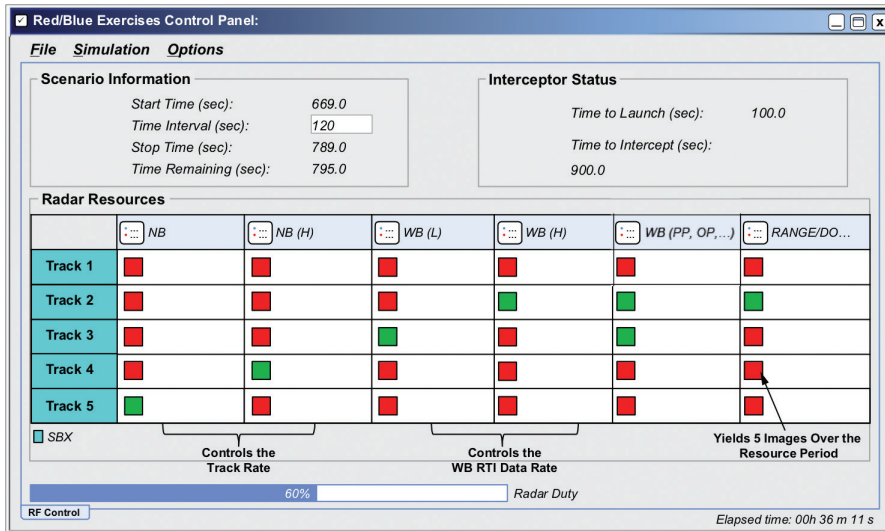
FIGURE 5. The radar control panel displays current status and waveform option buttons, including narrowband (NB) low-resolution waveform, wideband (WB) waveform, low pulse-repetition frequency (PRF) transmission (L), and high PRF transmission (H). Each option results in different levels of information quality. Green indicates that the sensor is going to employ that waveform on the given track, and red indicates that the sensor is not using the waveform on the given track.
