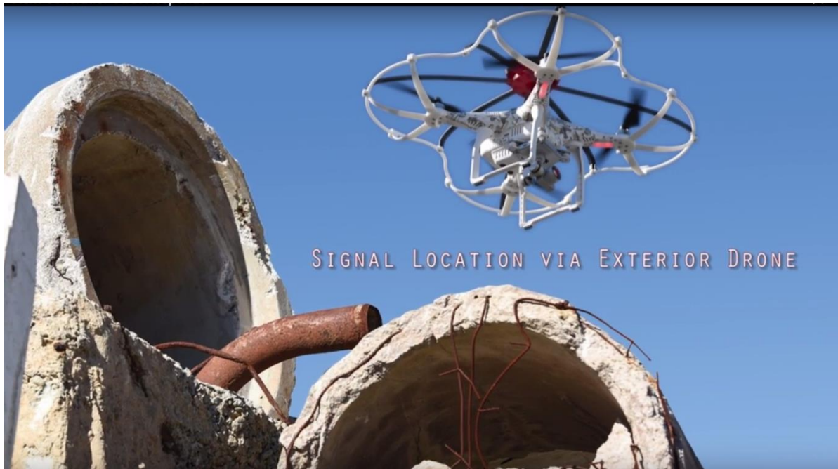
Figure C-3 Close-up of Lincoln Laboratory developed low-altitude UAS, seeking cell phone signals by flying low over building rubble.
