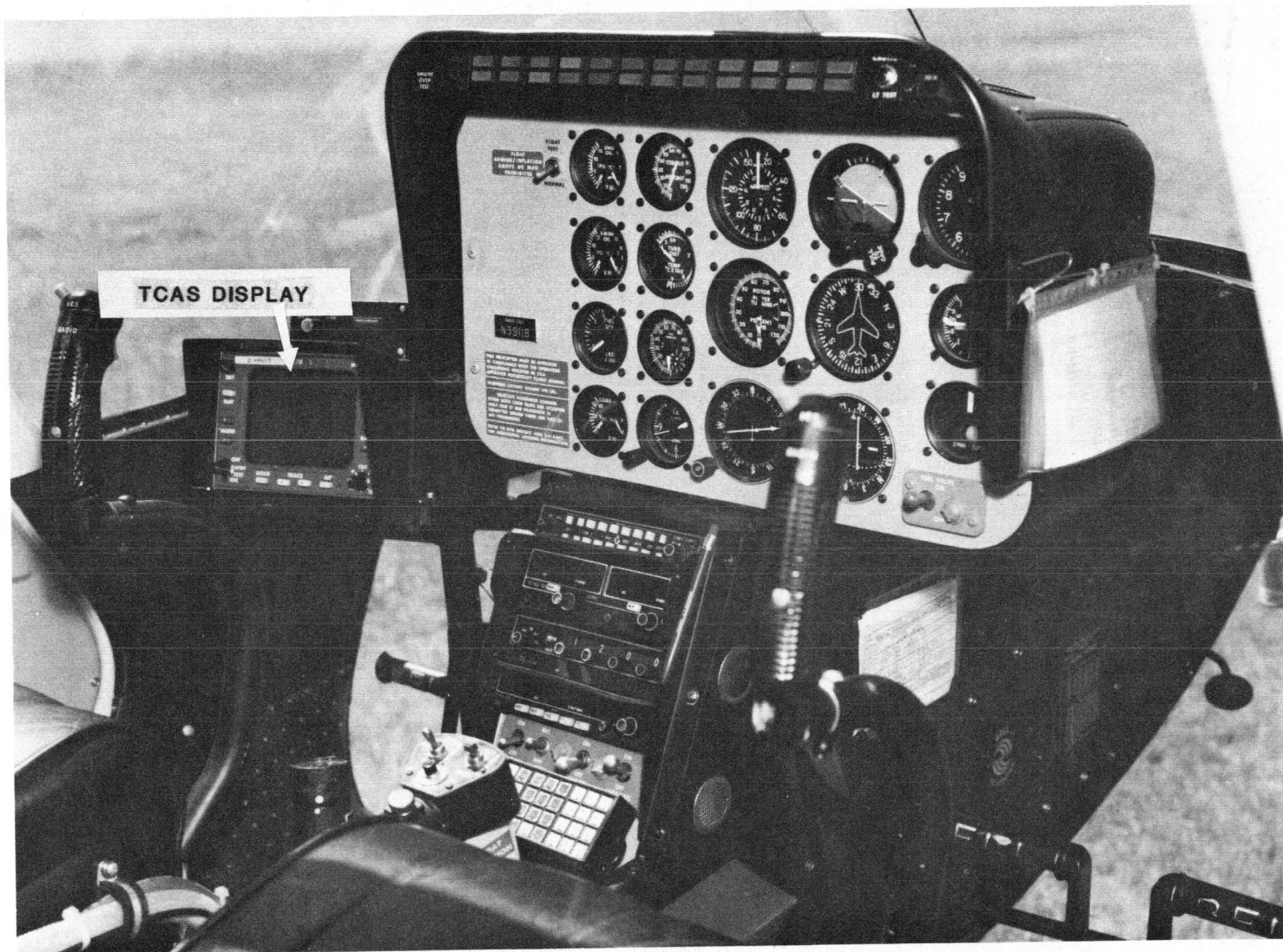
Fig. 1.2 TCAS display installed in the Long Ranger cockpit.
