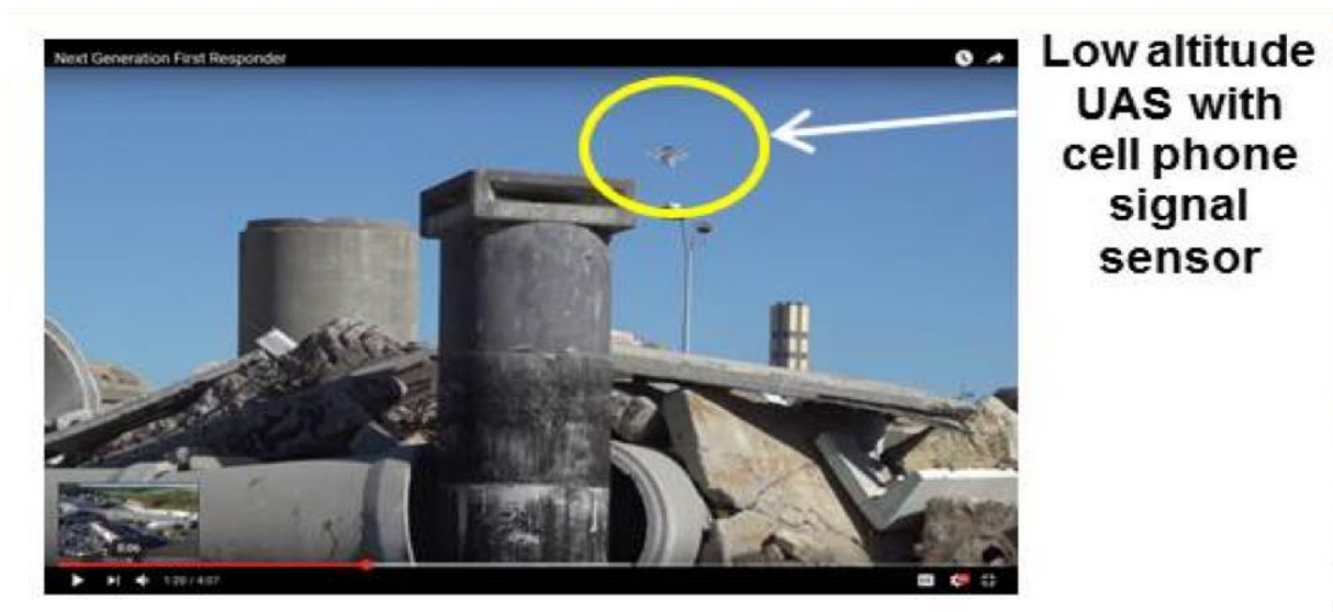
Figure C-4 Low altitude UAS searching in area of building collapse.
