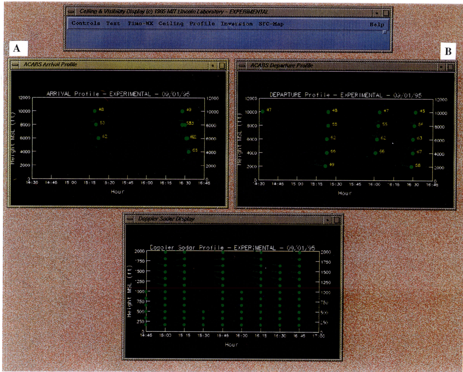
Figure 19. Vertical profile time-series displays from A) arrival aircraft reports, B) departure aircraft reports, and C) Doppler SODAR.
