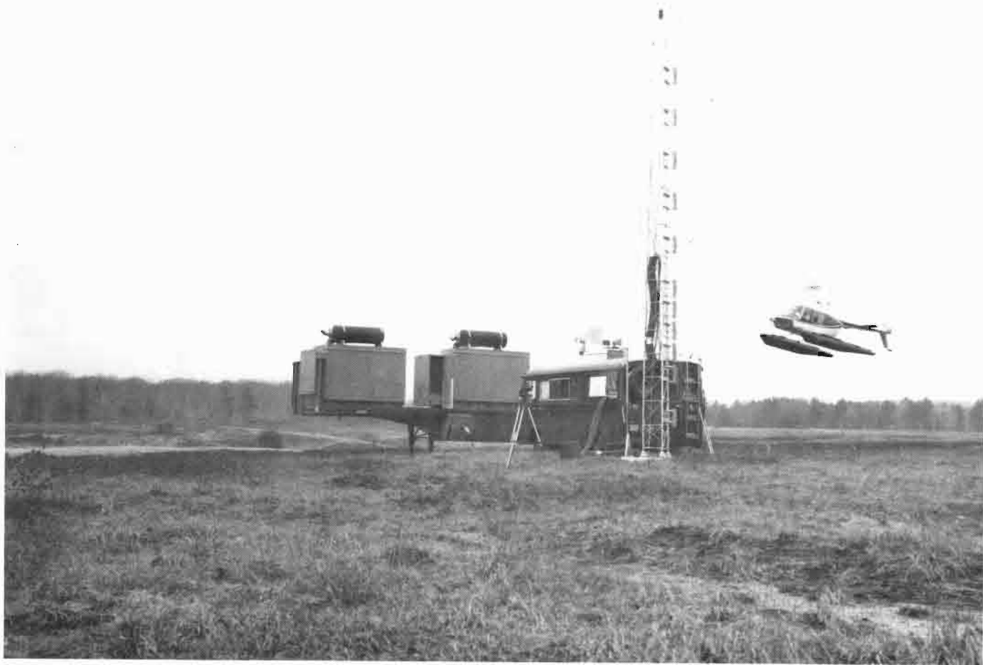
Fig.2-2. Experimental system for ground reflection data collection.
