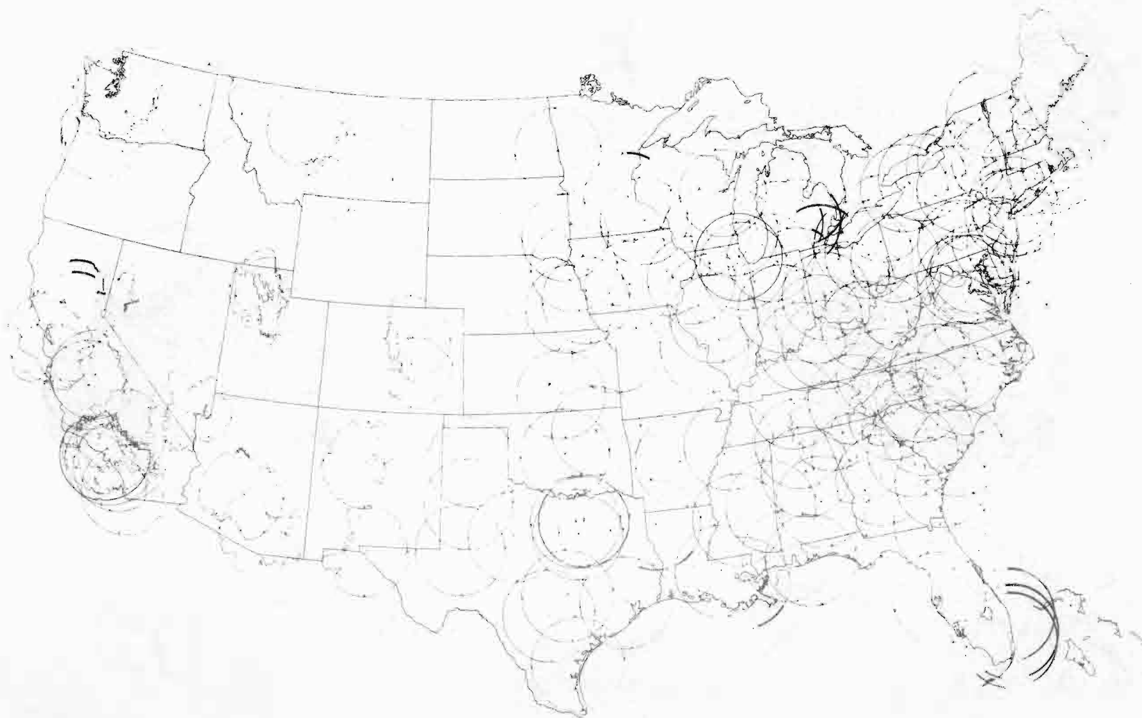
Fig. A.8. ASR composite coverage map, 15,000 ft. MSL, maximum range R_{\max} = 100 nmi.
