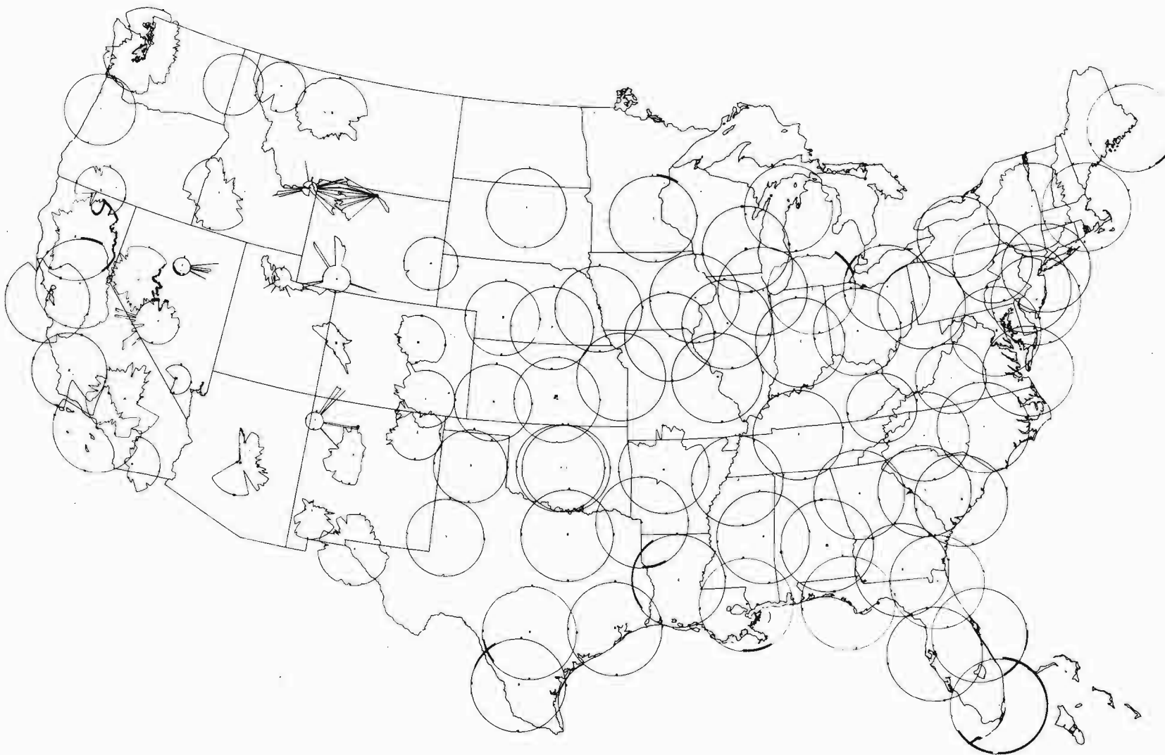
Fig. A.21. ARSR composite coverage map, 10,000 ft. MSL, maximum range R_{\max} = 100 nmi.
