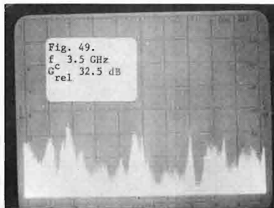
Figs. 47-50. Coaxial magnetron (QKH-1739LL) operated at 2.9 GHz (V-axis: 10 dB/div; H-axis: 100 MHz/div).
