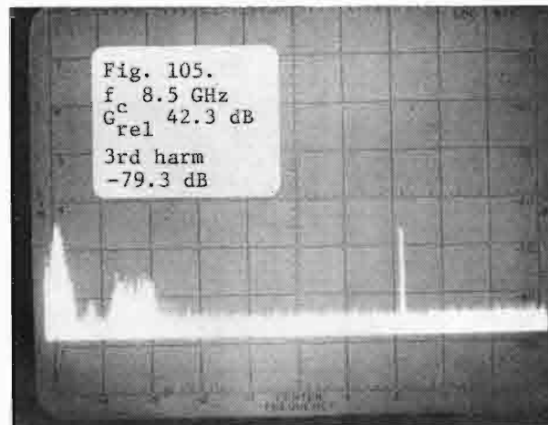
Figs. 102-105. Conventional magnetron (DX-276) operated at 2.9 GHz (V-axis: 10 dB/div; H-axis: 100 MHz/div).
