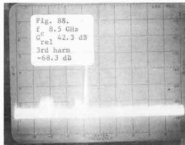
Figs. 85-88, Conventional magnetron (DX-276) operated at 2.8 GHz (V-axis: 10 dB/div; H-axis: 100 MHz/div).
