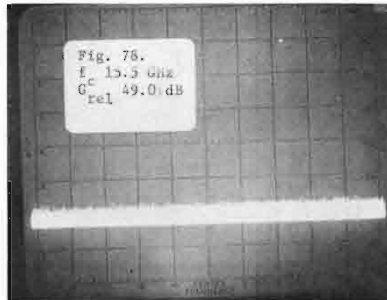
Figs. 76-79. Conventional magnetron (DX-276) operated at 2.7 GHz (V-axis: 10 dB/div; H-axis: 100 MHz/div).
