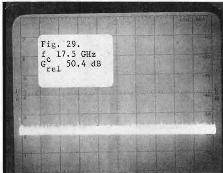
Fig. 29. Coaxial magnetron (QKH-1739LL) operated at 2.7 GHz (V-axis: 10 dB/div; H-axis: 100 MHz/div).
