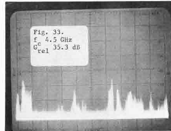
Figs. 30-33. Coaxial magnetron (QKH-1739LL) operated at 2.8 GHz (V-axis: 10 dB/div; H-axis: 100 MHz/div).
