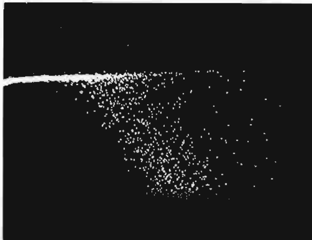
Fig. 118. Front edge of RF envelope - no priming (V-axis: linear power - not calibrated; H-axis: 10 nsec/div).
