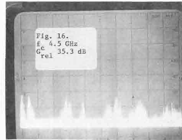
Figs. 13-16. Coaxial magnetron (QKH-1739LL) operated at 2.7 GHz (V-axis: 10 dB/div; H-axis: 100 MHz/div).
