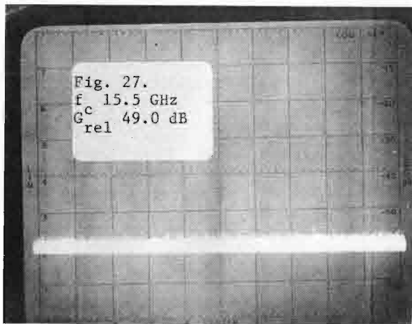
Figs. 25-28. Coaxial magnetron (QKH-1739LL) operated at 2.7 GHz (V-axis: 10 dB/div; H-axis: 100 MHz/div).
