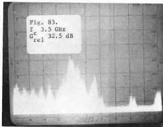
Figs. 81-84. Conventional magnetron (DX-276) operated at 2.8 GHz (V-axis: 10 dB/div; H-axis: 100 MHz/div).
