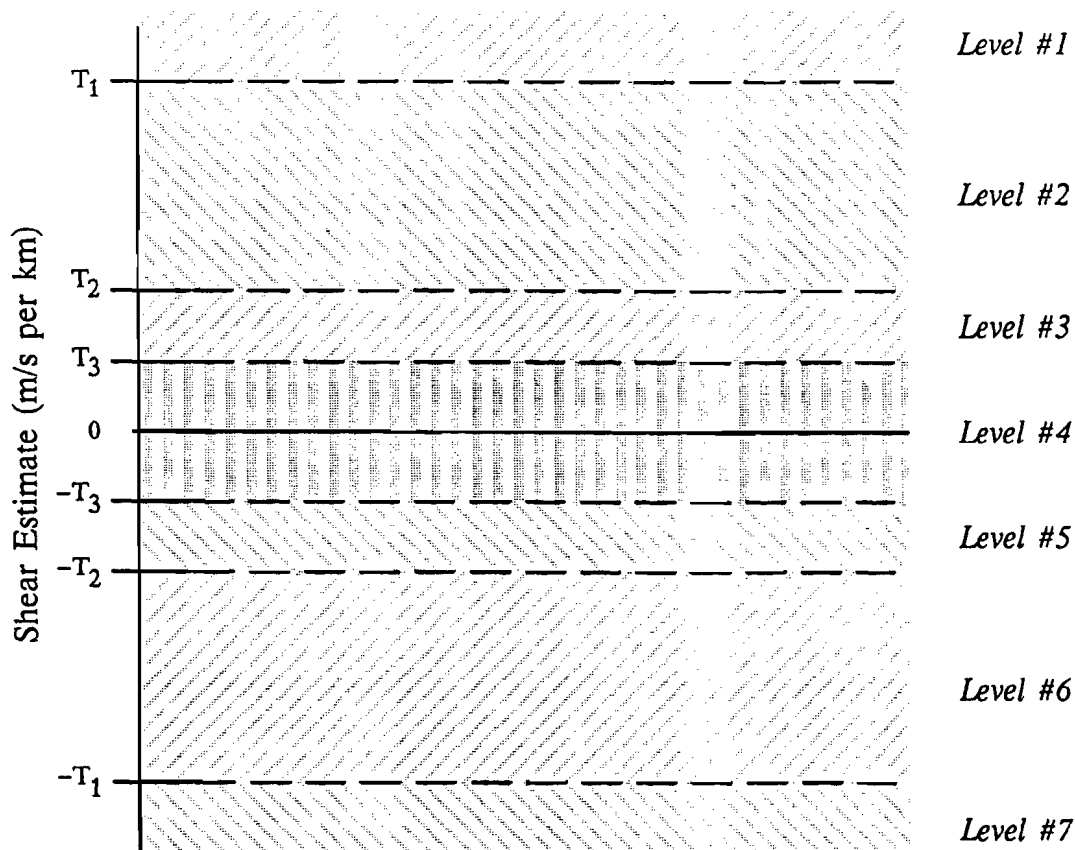
Figure 56: Quantization of shear values into seven levels. Three basic threshold parameters are applied to both positive and negative shear amplitudes, and the number of values for each region are tallied. The nominal values used for the three thresholds are 5, 3 and 2 m/s per km, respectively.
