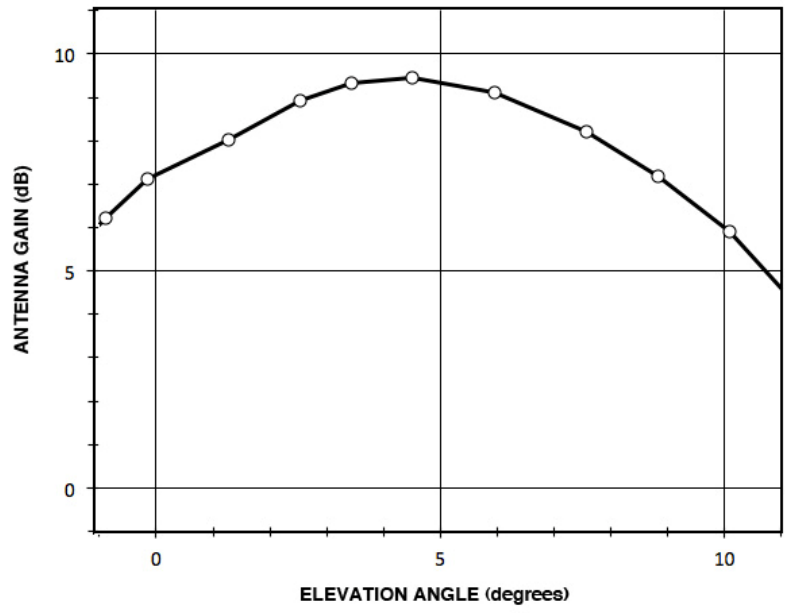
Figure 2. Elevation pattern of the omnidirectional antenna.
