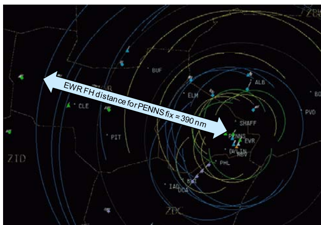
Figure 3-2. EWR TMA PGUI display showing the 390 nm FH distance for PENNS arrivals extends into western ZOB (just beyond Detroit [DTW] airport).
