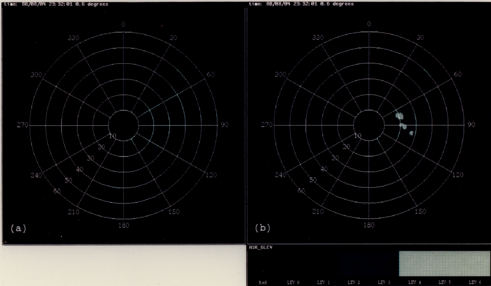
Figure 1. Simulated weather display from (a) current ASR systems and (b) ASR-9 weather channel (summation mode)
