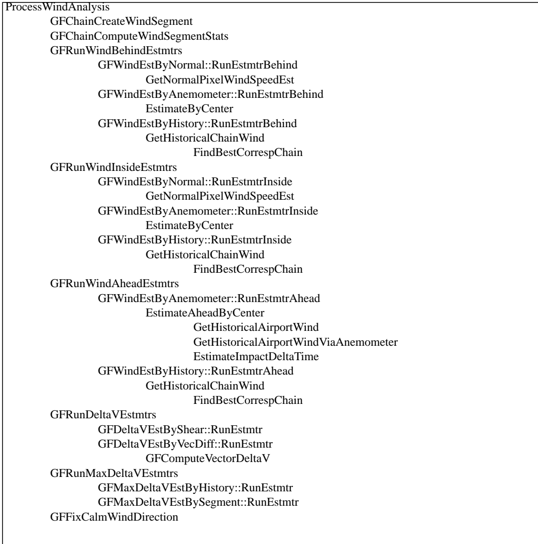
Figure 48. Function call tree for the MIGFA wind analysis stage (see text for description).
