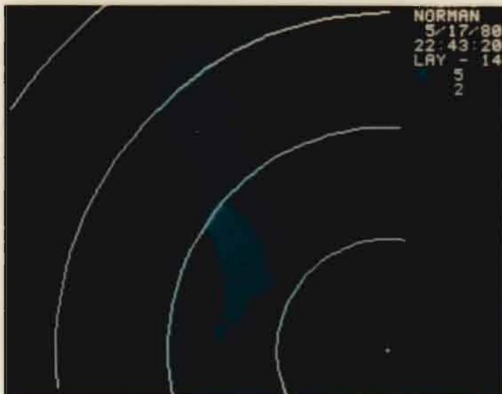
Figure II-7(a). Simulated ASR-9 six-level weather display on Air Traffic Controller's PPI. In "summation" display mode, all weather areas between a lower and upper threshold are shown with light intensity modulation. All weather areas above the upper threshold are shown with more intense modulation. Weather radar data are from the National Severe Storm Laboratory. Range rings are at 30 km intervals.
