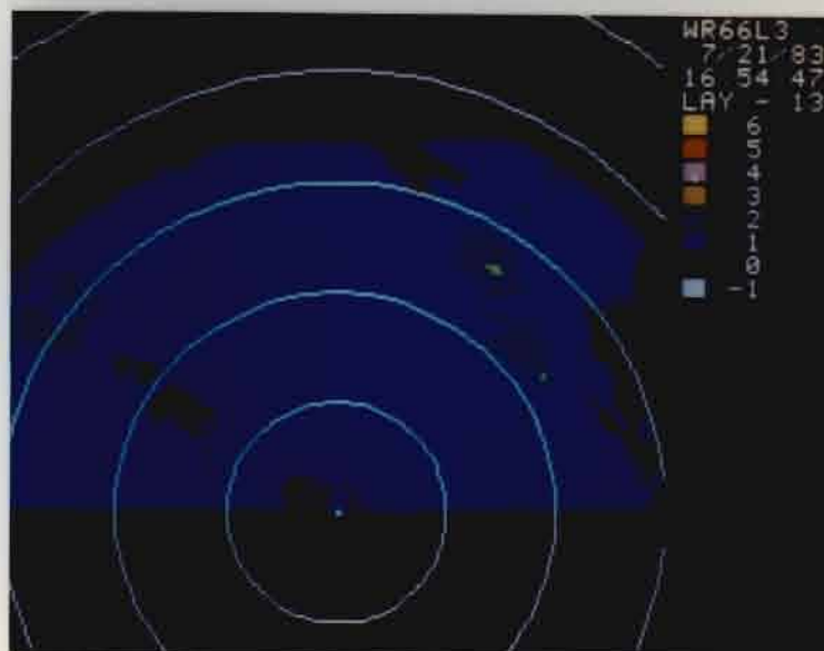
Figure V-14. (a) NWS levels corresponding to layer averaged reflectivity in the interval 0-12,000 ft. Range rings are at 30 km intervals. (b) Simulated ASR-9 report for 0-12,000 ft layer average. The dual beam estimation procedure described in the text was used. (c) NWS levels corresponding to layer averaged reflectivity in the interval 12,000 ft to echo top. (d) Simulated dual-beam ASR-9 report for 12,000 ft to echo top layer average.
