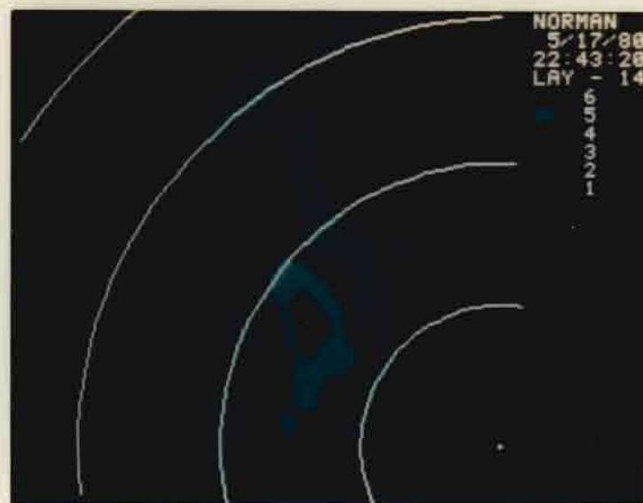
Figure II-7(b). Simulated example of "discrete" display mode on Air Traffic Controller's PPI. Two of the six weather levels are selected for display with two levels of brightness.
