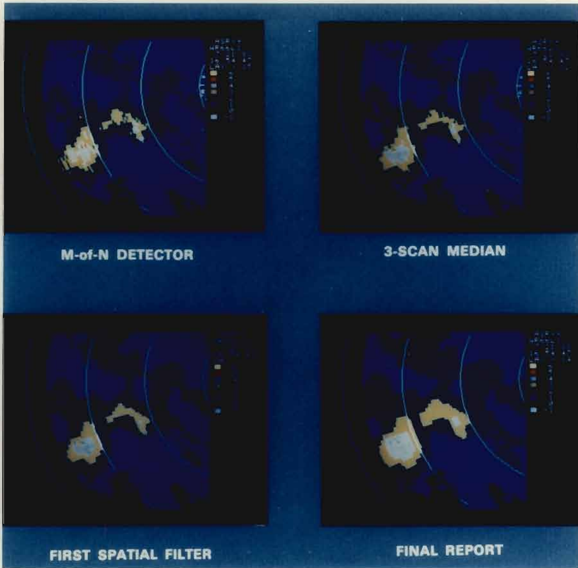
Figure IV-2. Simulated output of ASR-9 weather processor at outputs of M-of-N detector, 3-scan median filter, first stage spatial filter and second spatial filter. Range rings are at 30 km intervals from 30-120 km.
