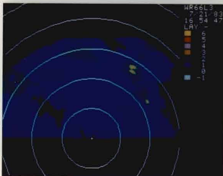
Figure V-14. (a) NWS levels corresponding to layer averaged reflectivity in the interval 0-12,000 ft. Range rings are at 30 km intervals. (b) Simulated ASR-9 report for 0-12,000 ft layer average. The dual beam estimation procedure described in the text was used. (c) NWS levels corresponding to layer averaged reflectivity in the interval 12,000 ft to echo top. (d) Simulated dual-beam ASR-9 report for 12,000 ft to echo top layer average.
