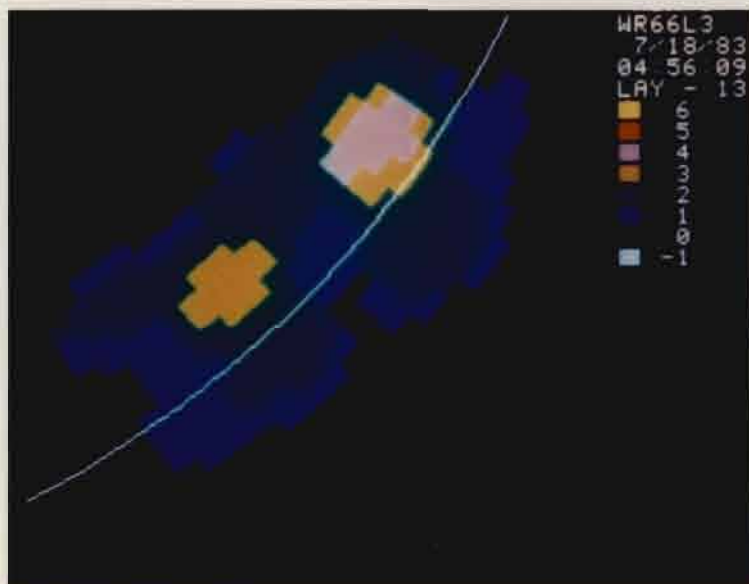
Figure V-6. (a) NWS levels corresponding to maximum reflectivity within ASR-9 resolution cells. Range ring is at 60 km. (b) Simulated ASR-9 report using threshold compensations plotted in Figure V-1. (c) Simulated ASR-9 report without threshold compensation.
