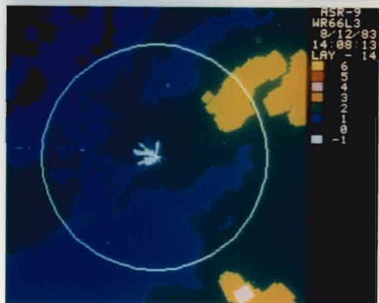
Figure IV-10 (Cont.). (d) Simulated output of the weather channel's M-of-N detector. (e) Simulation of smoothed, final report from weather processor. (f) As in part (e) except that ground clutter has been excluded from the simulation. (g) A simulated final report as in part (e) except that weather radial velocity has been set everywhere to 0 m/s and weather spectrum width to 0.75 m/s.
