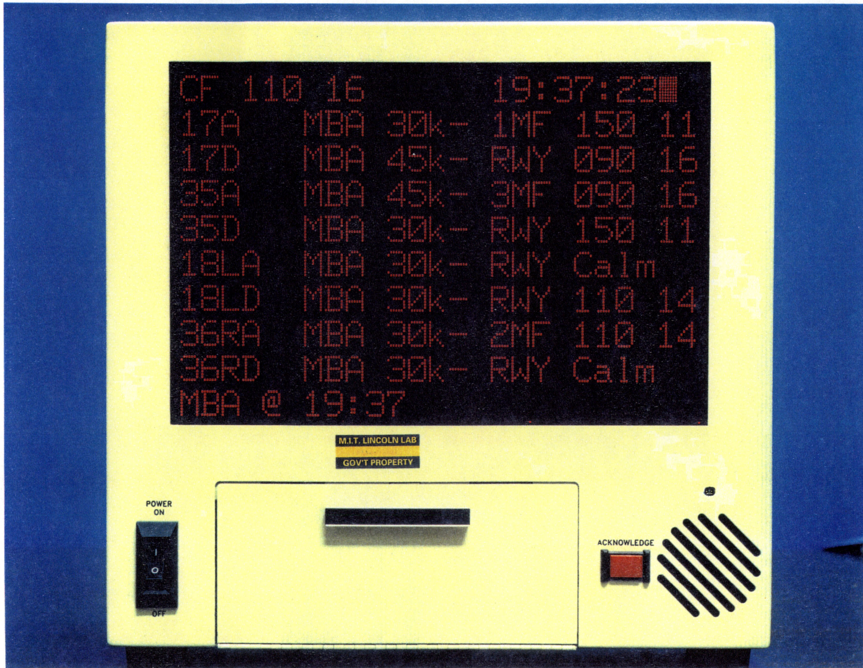
Figure 4b. Alphanumeric ("ribbon") display. The first line is read as "microburst alert on runway 17 arrival, 30 knot loss at 1 mile final, threshold winds 11 knots from 150 degrees."
