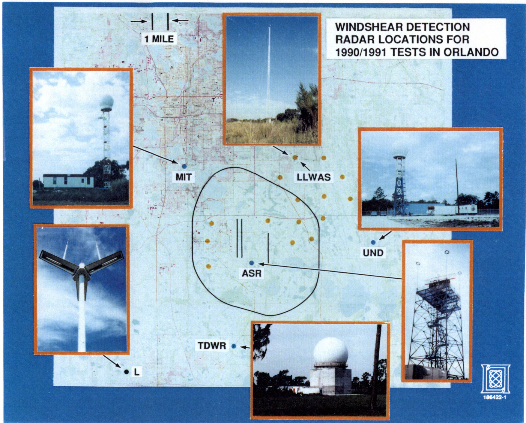
Figure 5. Map showing locations of Doppler radars, anemometers, and lightning detection system (L) relative to Orlando International Airport. The vertical black lines in the center of the picture are the three parallel runways at the airport.
