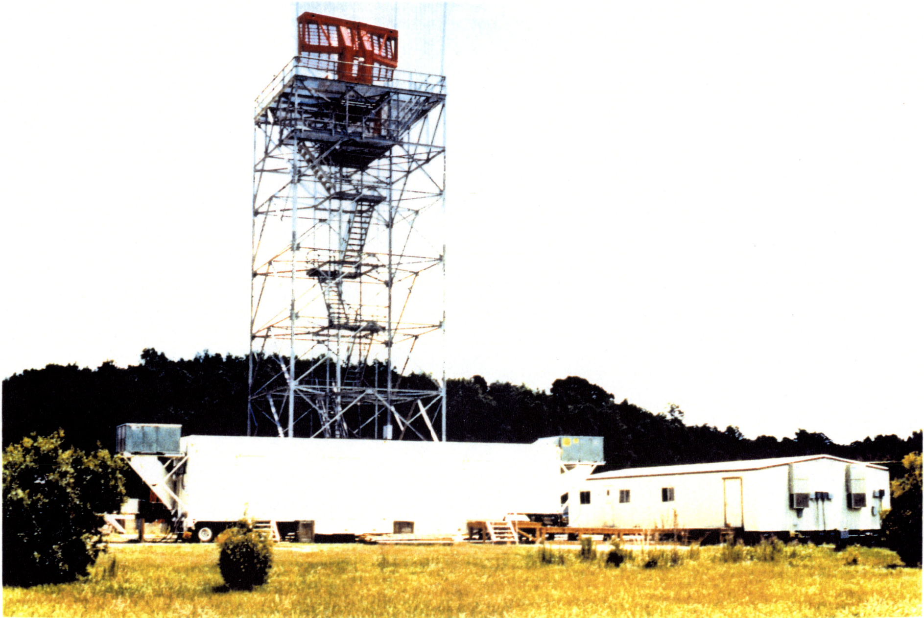
Figure 2. Photograph of ASR-9 Wind Shear Processor tested on Orlando International Airport.
