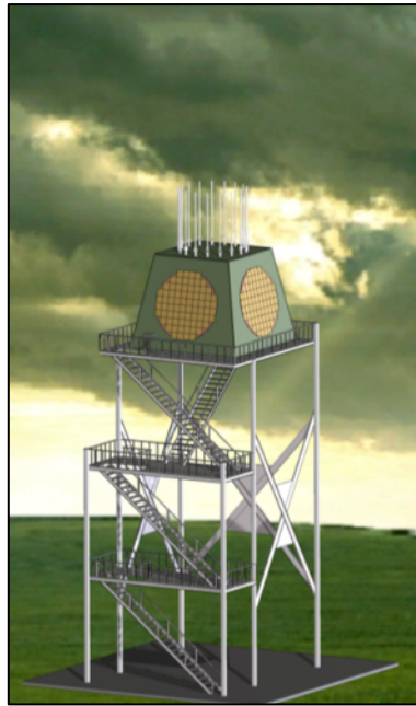
Figure 1-1. SSPAR array mounted on frustum of Terminal MPAR.
