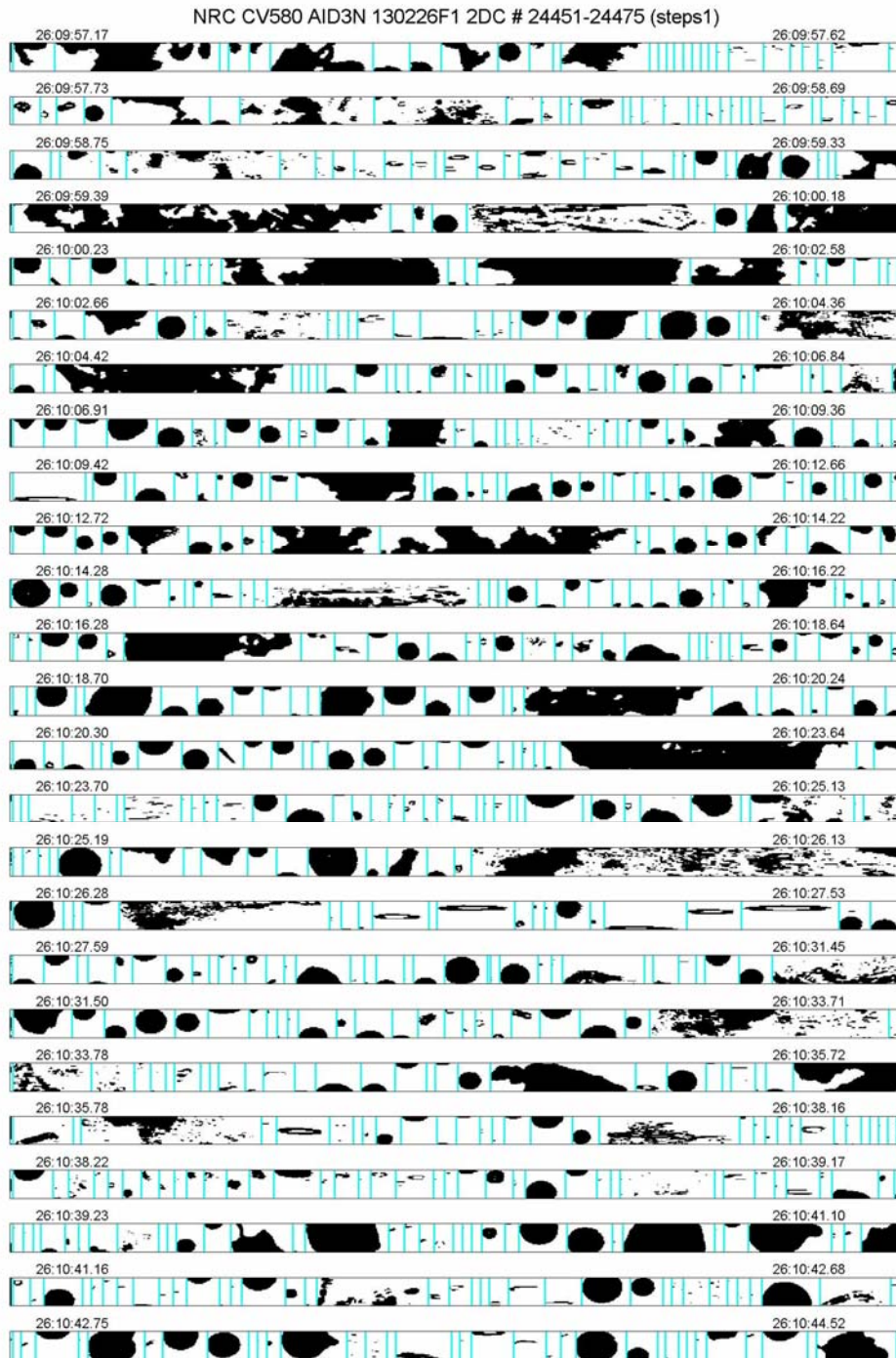
Figure 6-25. Imagery from the Particle Measuring Systems 2DC probe for the period 02:09:57 to 02:10:44 UT, showing an abundance of raindrops with sizes in excess of 1 mm diameter in a zone of freezing temperature ( T = 0^{\circ} to -4^{\circ} C).
