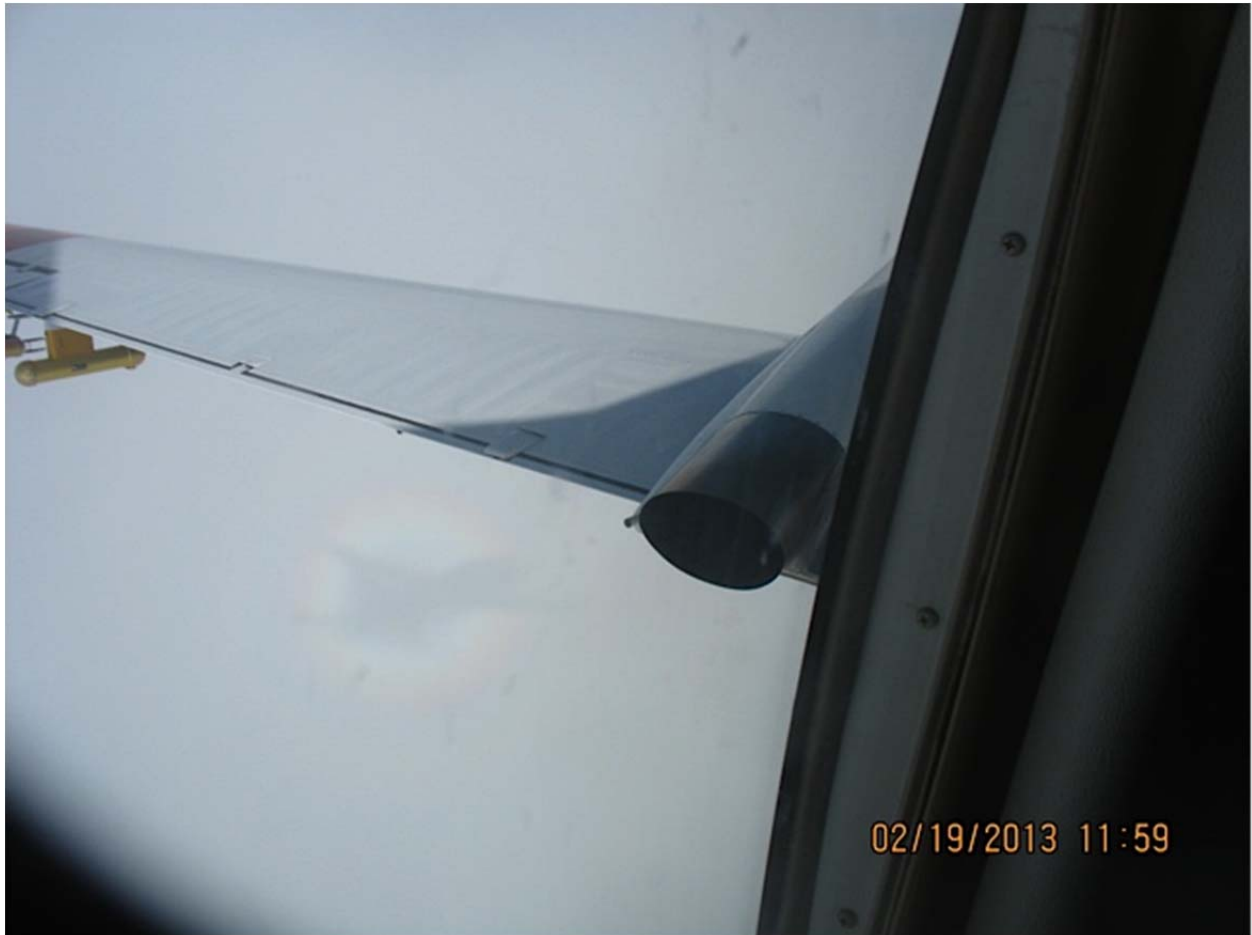
Figure 6-6. Documentation of the optical phenomenon glory in the cloud top when the aircraft exited into clear air near 4000 m. This observation of an upper cloud boundary at -20^{\circ} C is evidence in itself for the presence of supercooled droplets.
