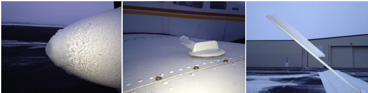
Figure 7-3. Photographs of rime accretion on the Piper Archer aircraft on (a) nose of aircraft, on (b) the gas cap on the wing, and (c) on the slanted antenna. These photographs were taken a few minutes after the plane landed.
