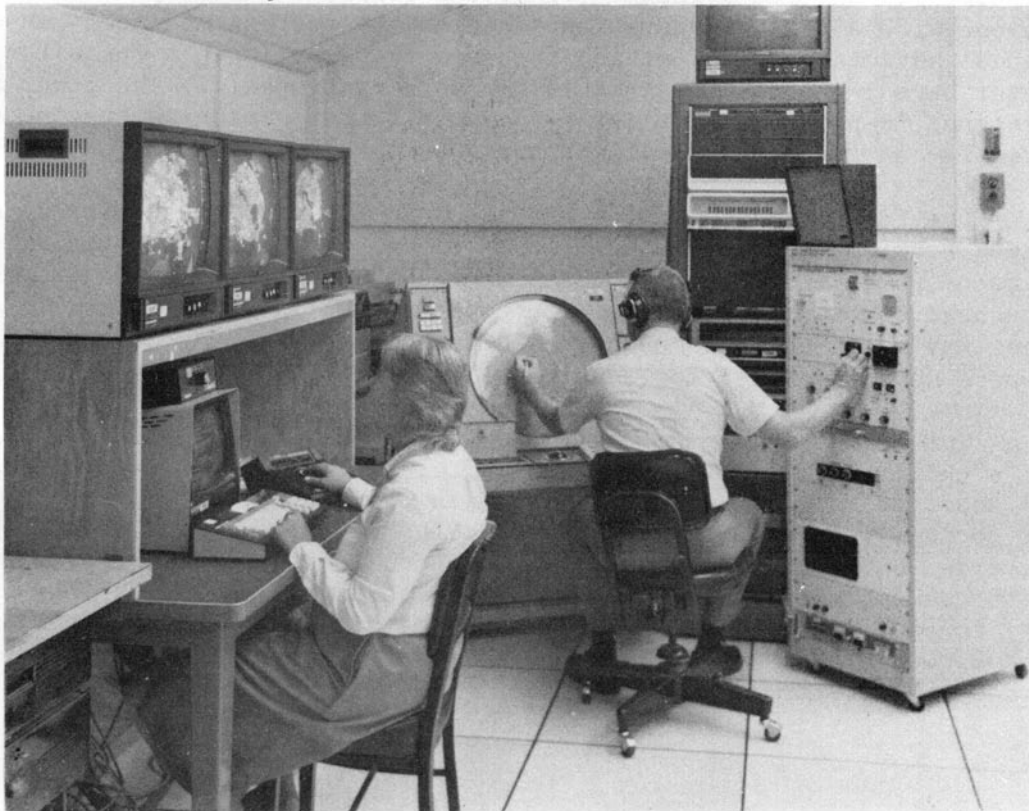
Fig. 1-6: Lincoln Laboratory Experimental Operations Control Center in Annex II. Radar data is being displayed on three monitors and radio operator is pinpointing aircraft on air traffic controller's plan view display.
