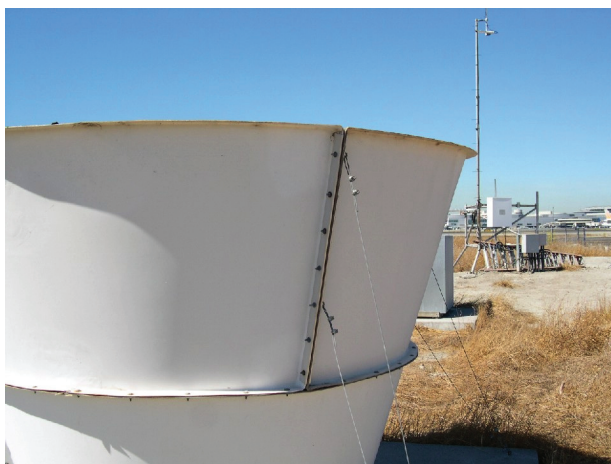
FIGURE 19. (left) Sensor field-site equipment at San Carlos airport. Foreground is a sodar baffle anchored to a cement pad. The background shows a tower mounted with sensors. (right) Sodar antenna viewed by looking down into baffle.
