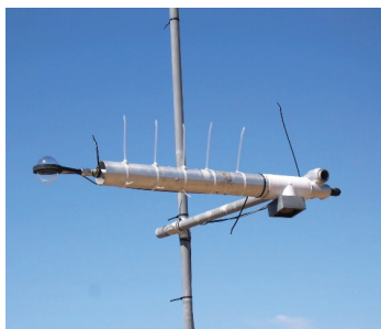
FIGURE 21. (left) Pyranometer system to measure incoming solar radiation, mounted on a tower. (right) Graphical representation of a solar radiation measurement (yellow curve) compared to the maximum theoretical solar radiation on a cloud-free day (red curve) for the sensor location and day of year. The blue line shows the ratio of measured/maximum radiation. This example shows stratus clouds clearing at approximately 1715 GMT.
