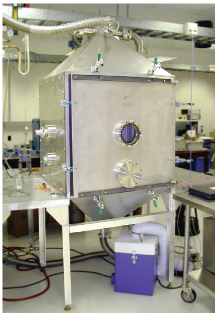
FIGURE 30. This laboratory aerosol chamber is designed to test aerosol sensors. It allows either the insertion of the sensor into the chamber or the ducting of aerosols from the chamber to the sensor. The aerosols enter the chamber at the top and are exhausted out the bottom through a HEPA filter.
