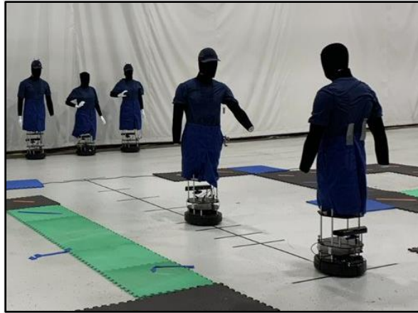
Figure 12. Mannequins with black RF-absorptive foam and phones placed in hip pockets, in ASDF test space.
