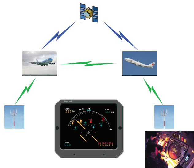
FIGURE 2. Automatic Dependent Surveillance—Broadcast (ADS-B)—driven technology still includes the air traffic controllers shown in the bottom right, but the information presented to the controller is obtained from ADS-B connections to global positioning sensors and ground-based transceivers. Aircraft that have ADS-B equipment can send and receive the same information directly to and from other similarly equipped aircraft and can observe all the information on nearby aircraft on the monitors in their cockpits (center).
