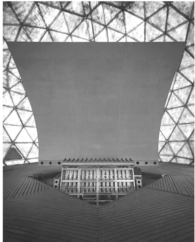
FIGURE 2. Sixteen-element linear-array test-bed facility at Lincoln Laboratory in 1960. Phased-array components such as antenna elements, low-noise amplifiers, intermediate-frequency amplifiers, mixers, transmitters, and beamforming techniques were tested in this facility.
