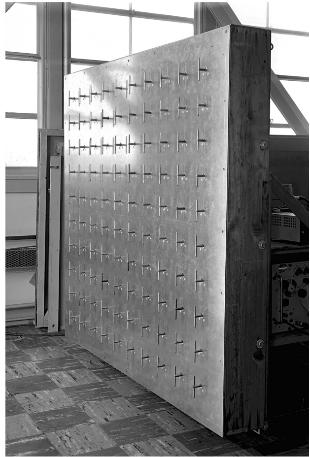
FIGURE 6. An early L-band dipole phased-array test bed developed by the Sperry Rand Corporation, used in Lincoln Laboratory array investigations during the 1960s.
