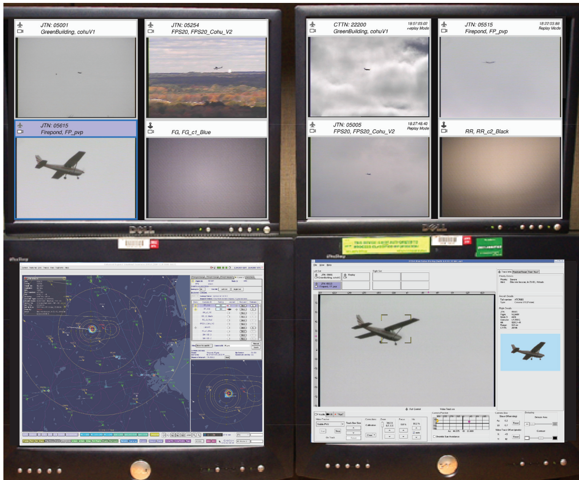
FIGURE 6. ERSA workstation. Four monitors show an array of images, including radar tracking and camera images. A single keyboard and mouse control the displays.
