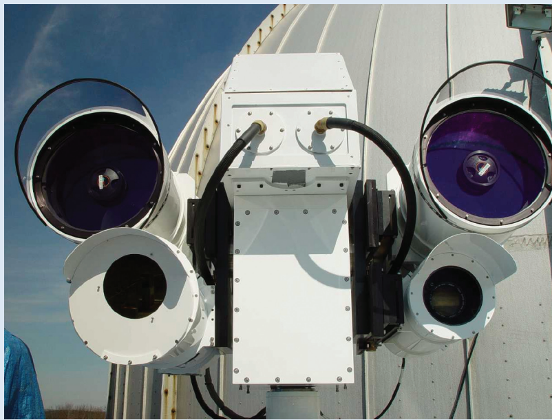
FIGURE A. Visual Warning System (VWS) node. Cameras are used to aim the VWS, and red and green lasers illuminate the target through 11 inch telescopes.
