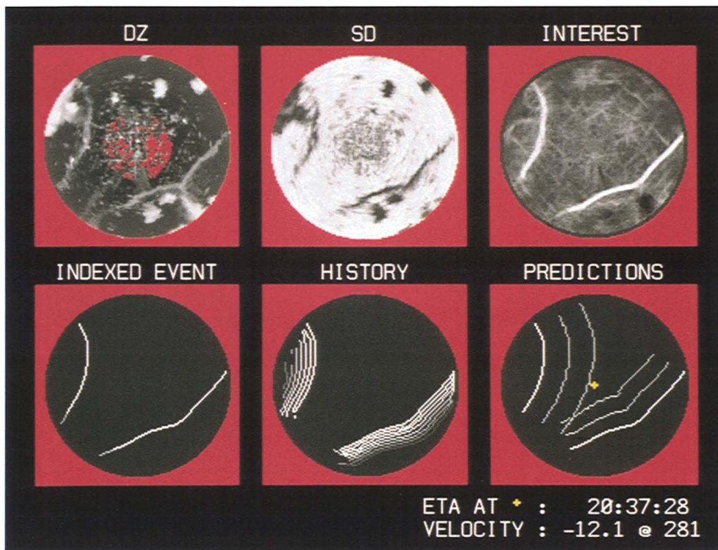
FIGURE 5. Processed scan summary. In the first row are the DZ (reflectivity) image, SD (standard deviation of velocity) image, and the combined interest image that has been computed from the DZ and SD images. The second row begins with the extracted indexed event. White pixels are those points which have been declared as part of a gust front. Gray pixels are those points which have not been tracked long enough to establish sufficient confidence. In the history frame, the current chain is shown in white and the preceding scans are shown in shades of gray (darker shades indicate more distant events in time). In the predictions frame, fat gray pixels indicate the 10- and 20-min forecasts of where the fronts are expected to be. Also shown at the bottom right corner are the estimated time of arrival of the next gust front to cross the radar site, the speed of the winds measured inside the front (in m/sec), and the direction (in degrees) from which the front is coming.
