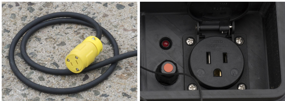
Figure 17. NEMA 1-15R ungrounded connector, which can be used directly with any MAPP AC interconnecting port (left), NEMA 5-15R as seen on the output enclosure (right).
