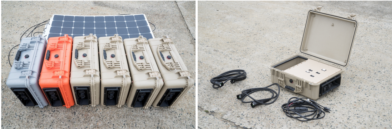
Figure 7. MAPP second year Phase 2 prototype: Grey output enclosure; tan (solar firmware) and orange (battery firmware) inverter enclosures and COTS PV panels. Interconnecting cable sets housed inside enclosures for transport.
