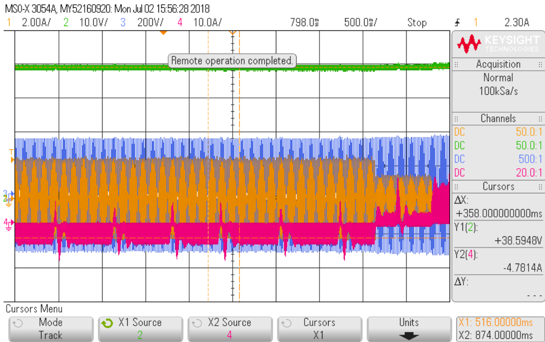
Figure 23. Battery supporting the load followed by load being removed and battery charging.
