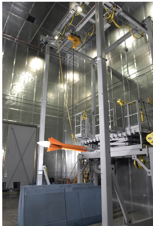
FIGURE 2. Gantry/crane system used in moving large test objects and support crew into the compact range chamber. The suspended object is a towed target frequently used for aircraft interceptor tests.
