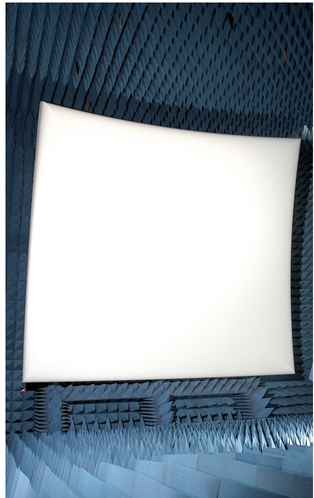
FIGURE 4. Photograph of the new 24 × 24 ft compact range reflector installed at Lincoln Laboratory. The reflector is a composite surface of several large machined panels that were hand-finished to the required tolerances before being coated with multiple layers of silver conducting paint and a final layer of white latex paint. The combined weight of the reflector and steel backup structure is approximately forty-four thousand pounds.
