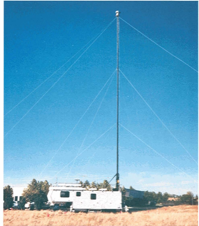
FIGURE 7. Measurement van used to assess the suitability of potential TDWR sites. Shown with its RF masthead installed, the van collected data to determine the LOS coverage, RF interference, and local-area ground-clutter values at the candidate locations for the TDWR systems.
