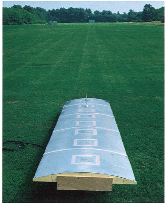
FIGURE 3. TCAS antenna measurements at the Lincoln Laboratory Antenna Test Range (ATR). In the foreground, the TCAS antenna and VHF blade antenna are mounted on a mock-up of a Boeing 727 fuselage. During the experiments, the fuselage was mounted in an anechoic chamber (Figure 4). At the far end of the range is the dish antenna that provides the signal source used for the bearing-error measurements.
