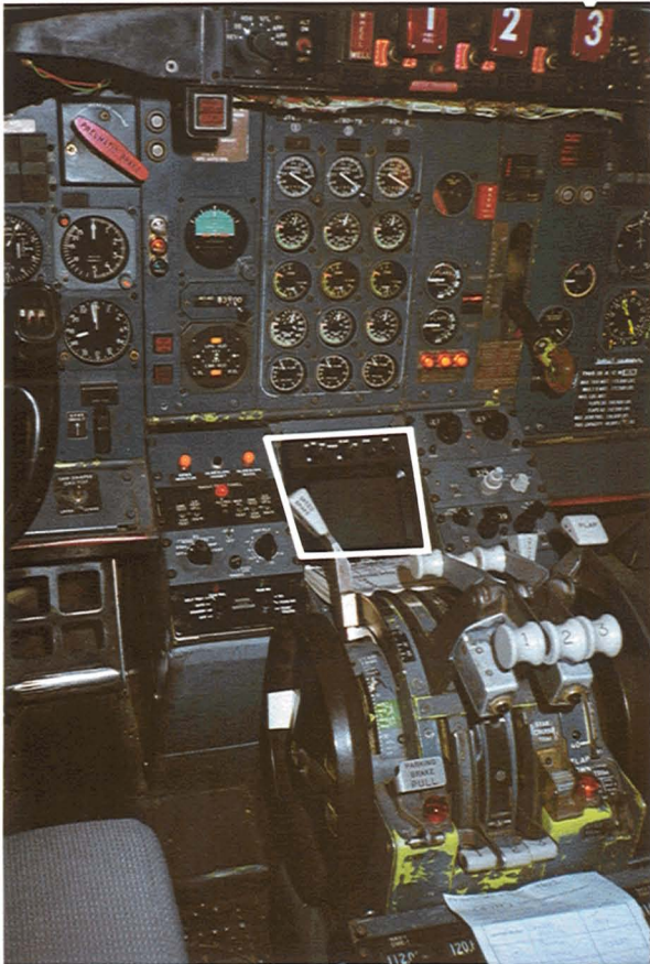
Fig. 11—Operational testing in a Boeing 727 operated by Piedmont Airlines. The cockpit photograph shows the traffic advisory display.
