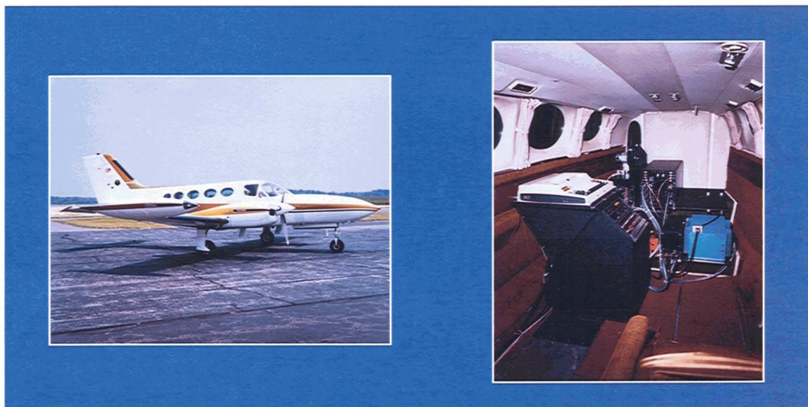
Fig. 8—Lincoln Laboratory TCAS Experimental Unit. This equipment, installed in a Cessna 421 twin-engine aircraft (left), was operated by Lincoln Laboratory for TCAS experiments, measurements, and the early pilot tests.
